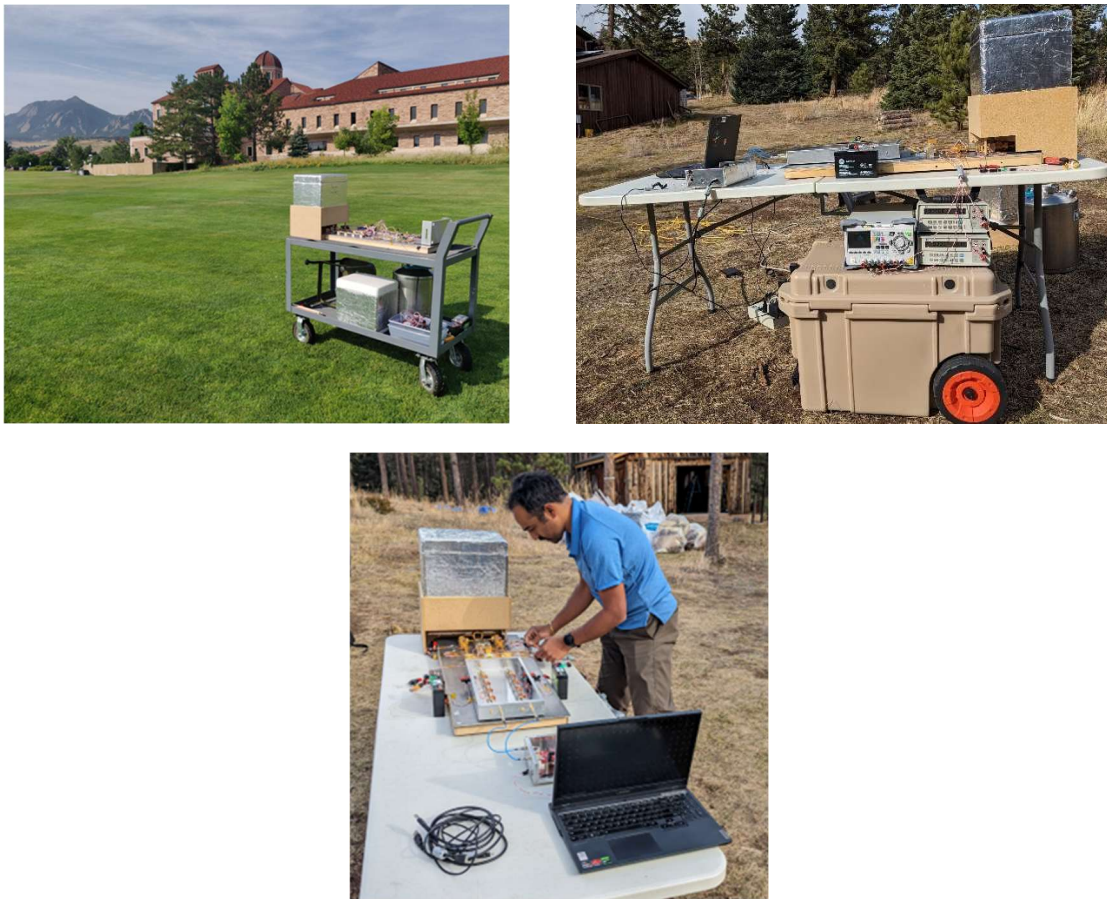
Figure 7.2 Outdoor Sky measurements with 2SQCC spectrometer (top - left & right). Aravind Venkitasubramony performing the pre-measurement sanity checks and getting the instrument ready for measurements (bottom).
