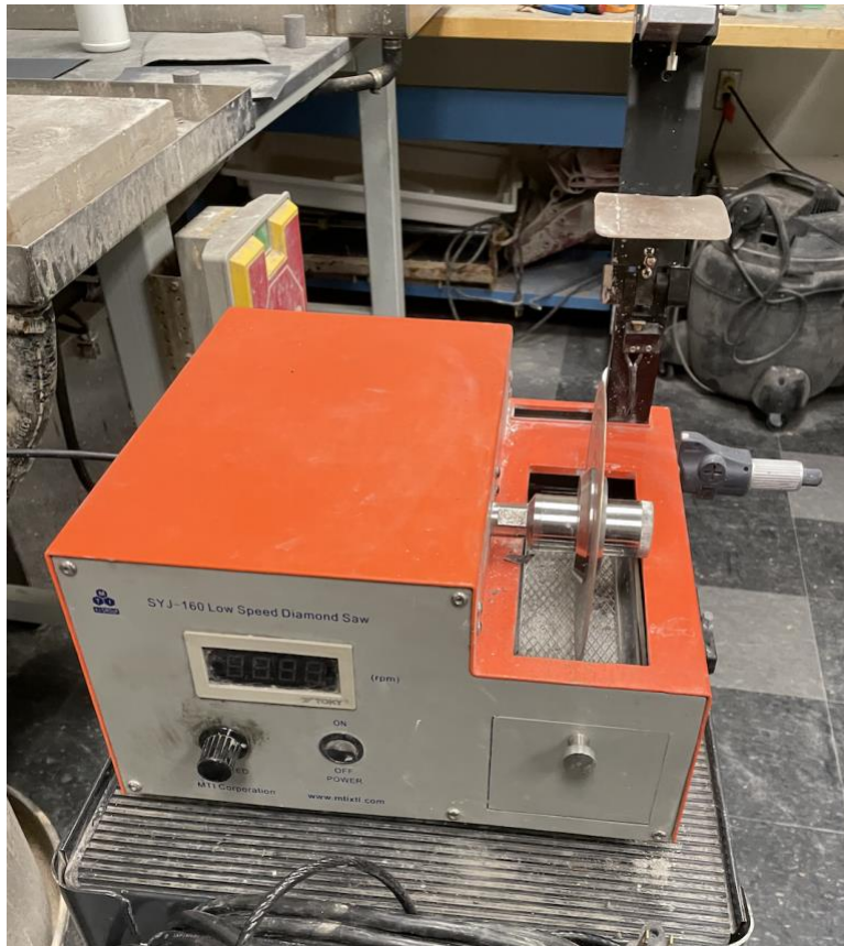
Figure 6.5: Image of saw used to reduce length of vertically bedded specimens for permeability testing
