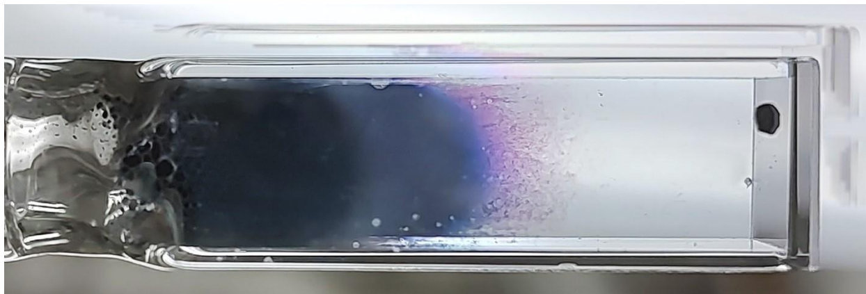
Figure 2.6: Potassium mirror deposited on the inside of cuvette with gradient of potassium metal thickness. The thinnest part of the mirror shows individual particles of potassium.
