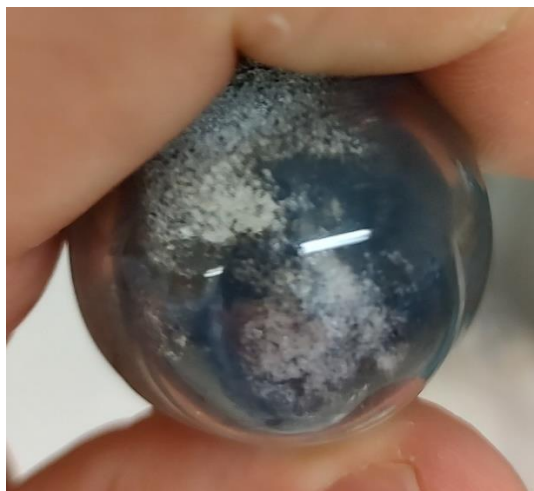
Figure 3.7: K_1 : p -terphenyl, showing islands of unreduced p -terphenyl.
