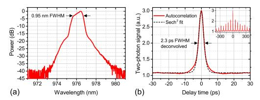
Fig. 2. (a) Optical spectrum of the laser source. The spectral bandwidth is 0.95 nm (-3 dB). The resolution bandwidth of the optical spectrum analyzer was 0.08 nm. (b) Autocorrelation of the laser source fitted to a sech<sup>2</sup> pulse shape (dashed line). The wings of the pulse indicate uncompensated higher order dispersion. The extended autocorrelation (inset) shows the burst duration of  $\sim 100$  ps. Pulse bursts include several pulses of 2.3 ps duration.
