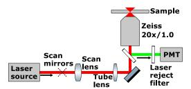
Fig. 3. Two-photon laser scanning microscope schematic. The laser beam is scanned across the sample using galvonometric mirrors and the combination of scan and tube lenses. The microscope objective focuses the excitation laser and collects the fluorescence light. Fluorescence is separated from the excitation laser using a dichroic mirror and color filter and detected using a photon-counting photo-multiplier tube (PMT).
