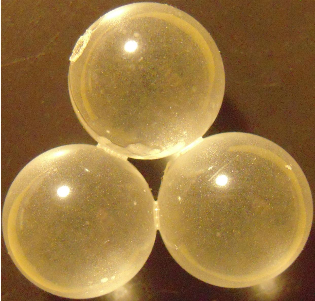
Fig. 4.1: The experimental agglomerate of three, acrylic Spheres (touching), with a dimensional sphere radius  $a_s \approx 0.95$  cm. Since  $a_s/b_s \approx 6.46$  for three touching spheres, the radius of the circle that just touches each sphere at the mid-plane location within the constriction is  $b_s \approx 0.15$  cm.
