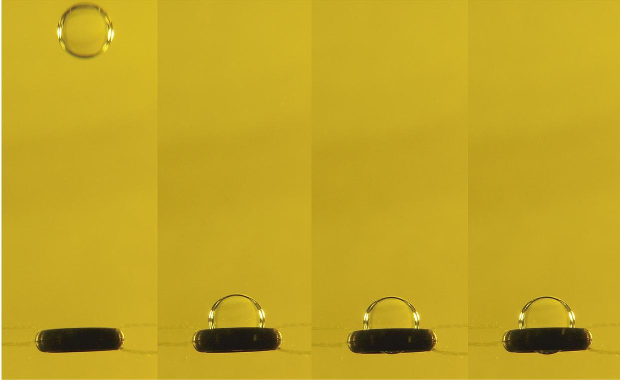
Fig. 4.3: Experimental stills of a 100% water drop being trapped in an O-ring constriction with  $a/b_s = 1.22$ ,  $a_s/b_s = 0.567$ ,  $\mu_d/\mu_e = 0.013$ , and  $B = 0.21$ ; the first three drop stills were taken about 2 s apart, and the last still was taken after a 20 s interval.
