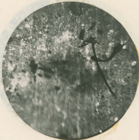
Figure 4.--Photomicrograph of Dunnet shale (x150), showing carbonized fragments.
