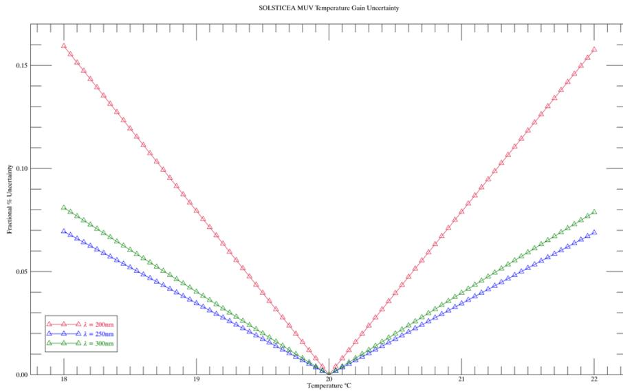
Figure 10: Temperature gain uncertainty as a fractional percentage of temperature gain vs. temperature
