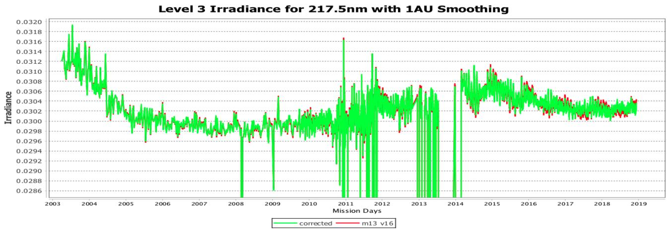
Figure 8: Example time series at 217.5nm showing the spot-size corrected irradiance.
