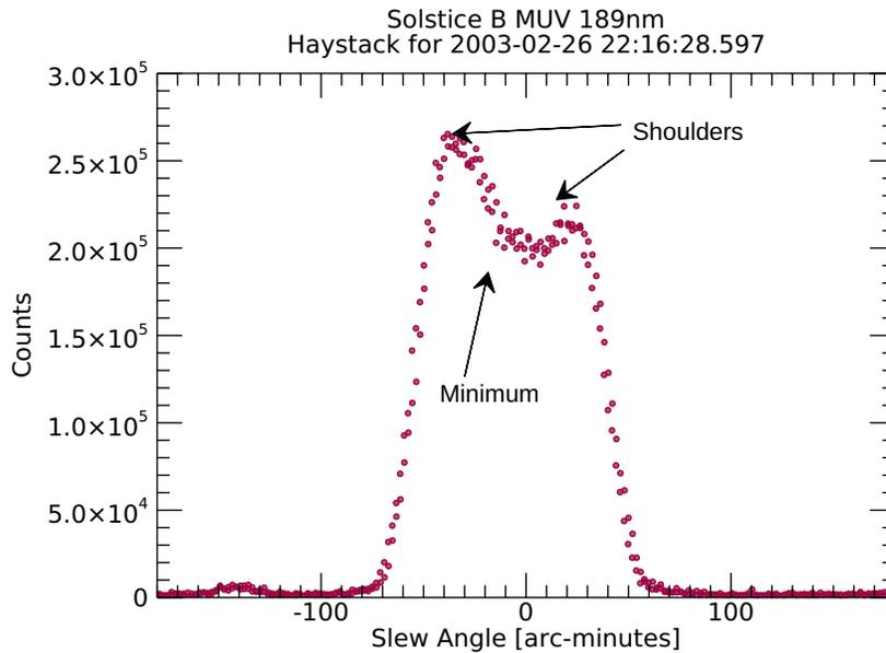
*Figure 1: Cruciform alignment "haystack" scan at 189nm*
