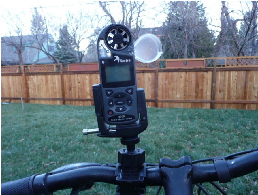
Fig. 3. The Kestrel 4000 Weather Station on a bicycle-mounted platform.
