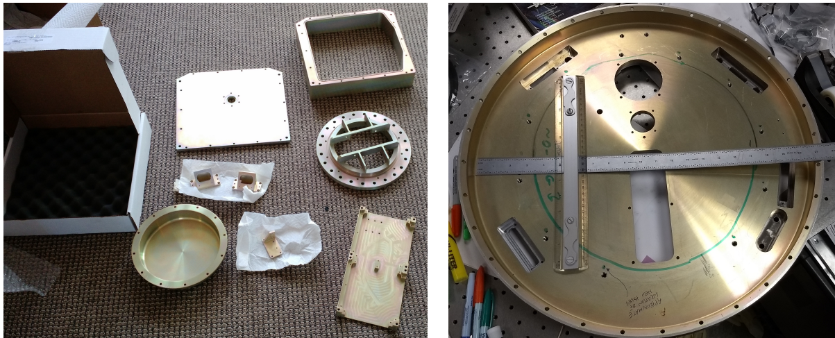
Figure 2.20: Two photos (out of many) of the payload build up. Left: Newly arrived parts are inspected after having been iridited. Right: Adjustments to the spectrograph bulkhead are calculated after a machining error resulted in an O-ring groove design not functioning in the assembled payload.
