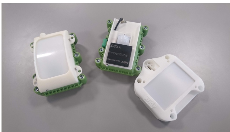
Figure 3. The original passive latrine use monitor (PLUM) design (left) was modified with a laser-cut custom bracket and industrial 3D-printed enclosure (right) to incorporate a RFID reader and tamper-resistant mounting system.
