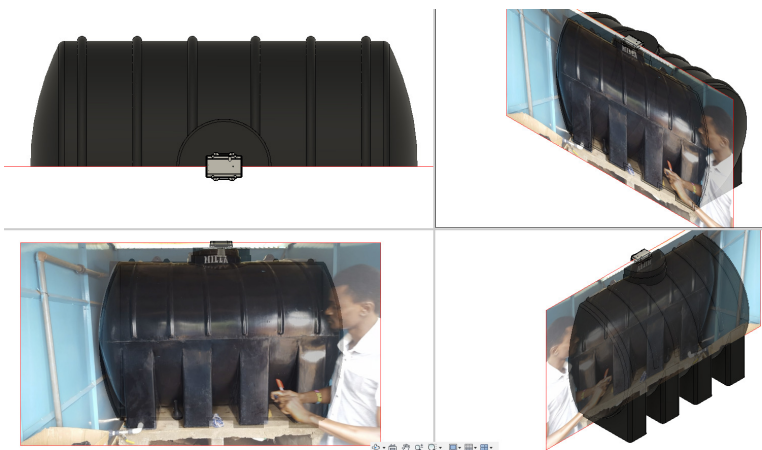
Figure 5. Collaborator feedback is crucial to effectively using remote design to improve early product prototypes. In this case, collaborators provided a few photographs and hand measurements to allow the design team to develop a virtual kiosk cistern prior to deployment.
