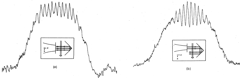
FIG. 1. (a) Ramsey pattern obtained for the P(4) F_1 \text{SF}_6 line with three standing waves (interaction geometry illustrated by the inset). The horizontal scale is linear in frequency and one fringe period corresponds to 94 kHz. The laser power was adjusted for optimum fringe contrast. The signal was recorded in a single one-minute sweep with a 0.1 s time constant and a 30 Hz modulation frequency of the laser amplitude. (b) Same as (a) with four traveling waves.
