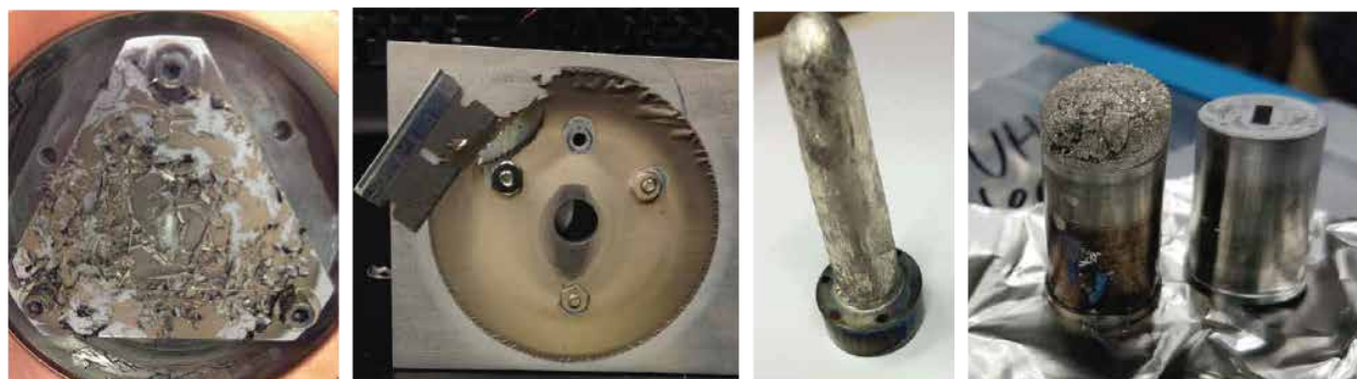
Figure 4.14: A variety of the types of clogging experienced by our calcium system both on the oven nozzles and on the atomic beam collimation apertures.
