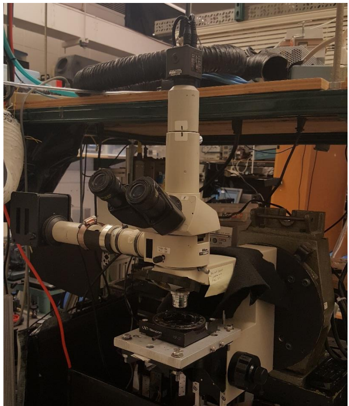
Figure 7: Nikon Optiphot Microscope and Goniometer. The microscope has a Watec camera mounted on the top and an incandescent light source mounted on the arm to the left. The entire microscope is attached to a goniometer, seen at the rear of the microscope.
