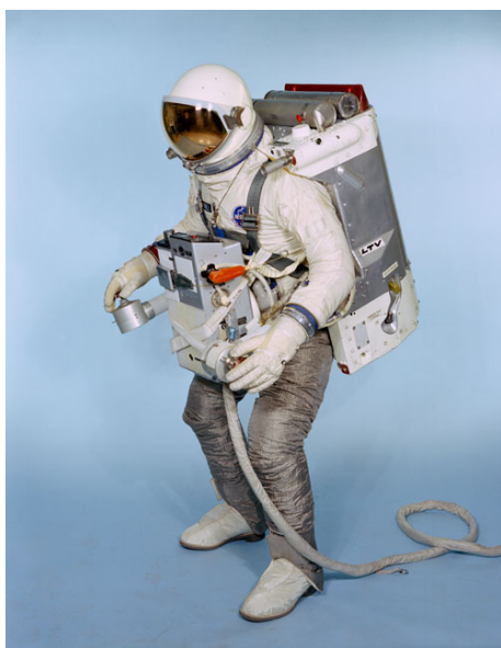
Figure 2.2. The Gemini AMU (Astronaut Maneuvering Unit), first developed for the MOL. Source: NASA
