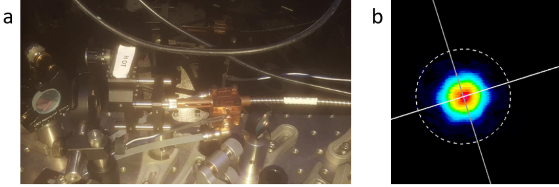
Figure 2.14: The hollow-core photonic crystal fiber. (a) The brass cooling block attached to the fiber connector, and the coupling optics for the fiber. (b) The profile of a focused beam far from the fiber output. Note the hexagonal shape caused by the core structure of the fiber. Any aberrations wash out the corners.
