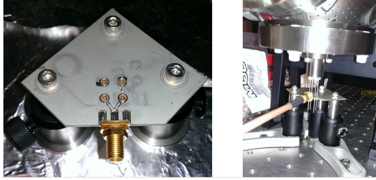
Figure 8.22: A PCB designed to couple the AC signal into the transmission line. The left image shows the PCB whose four holes go around the four feedthroughs, and the right image shows how it all looks when connected together.
