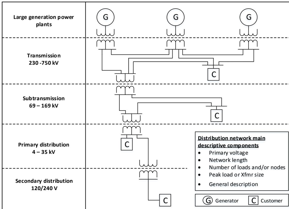
Figure 1. Power system infrastructure grouped by voltage levels.
