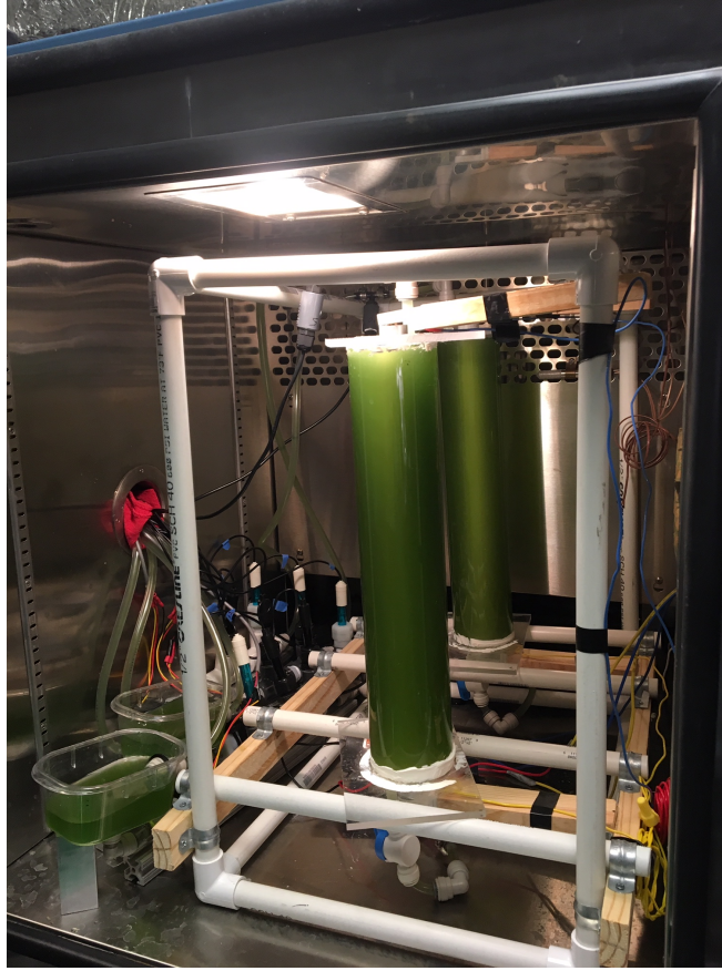
Figure 73. Vertical tubular bioreactors filled with dense culture, placed in environmental chamber. Start of long-term culturing experiment. Lighting at the top of the environmental chamber is for photographic clarity only and were turned off during the experiment.
