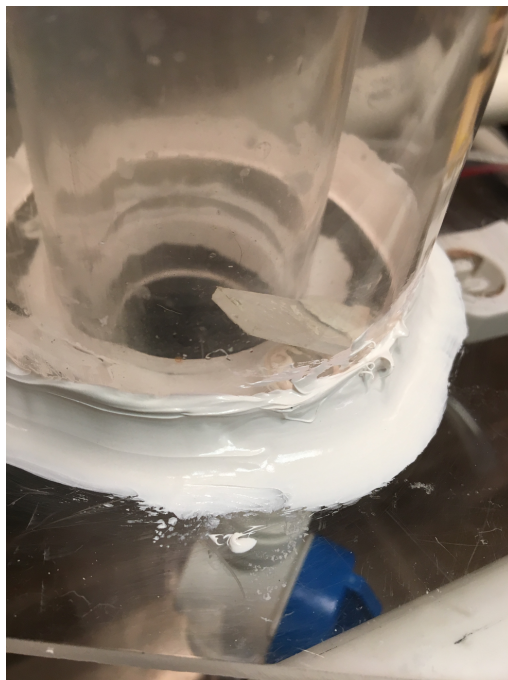
Figure 72. Plastic vane glued to bottom of acrylic annulus, over the inlet port (boxed).
