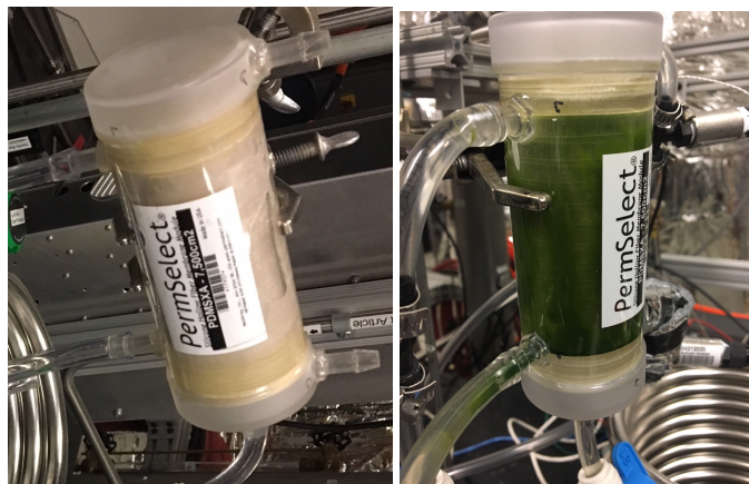
Figure 77. The nonporous membrane actively filtered out cells from the photobioreactors. New membrane before the start of an experimental run (left) and the same membrane at the end of the 25-day trial (right).
