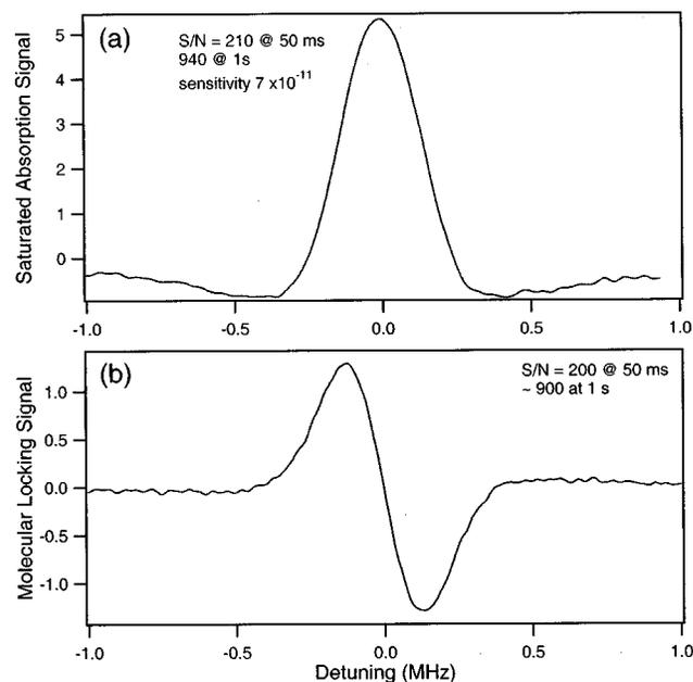
Fig. 5. (a) Intracavity saturated absorption signal of  $C_2H_2(3\nu_3)R(29)$  transition at 1031.653 nm, with 3-mTorr sample gas; saturated absorption, 0.07 ppm; FWHM  $\sim 500$  kHz. The detection sensitivity normalized to 1 s is  $6.4 \times 10^{-11}$  of the integrated absorption. (b) Antisymmetric error signal derived from the same molecular transition that is used to stabilize the laser-cavity system.
