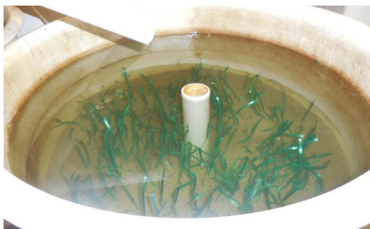
Figure 7. Two circular tanks contained simulated Zostera marina meshes weighted with rebar and covered with 1-5 cm of sand. The green polypropylene ribbons attached to the meshes were pulled up from underneath the sand.
