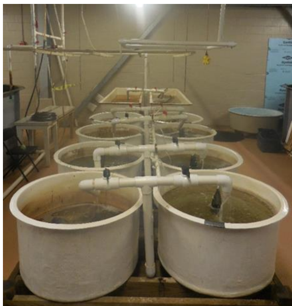
Figure 5. Flow-through seawater system in the Seawater Research Lab at VIMS. Water was pumped from the York River, filtered, and distributed to each tank through pipes. Six circular tanks were used for trials. One held juvenile blue crabs, and one held striped burrfish. One long rectangular tank held adult blue crabs.
