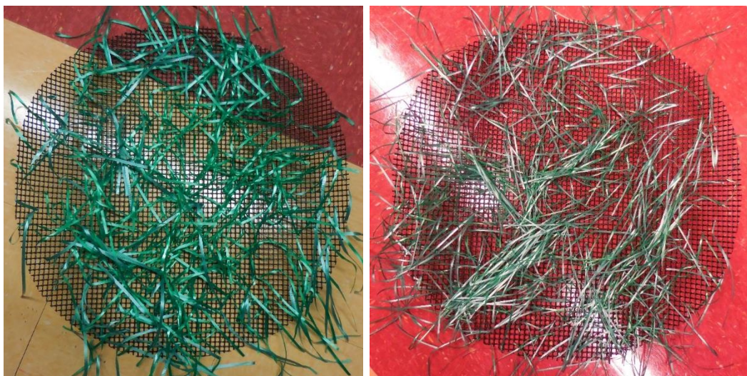
Figure 4. Artificial seagrass meshes of Zostera marina (left) and Ruppia maritima (right). Green polypropylene ribbons 20-cm in length were tied to black circular Vexar meshes (0.283 m 2 ).
