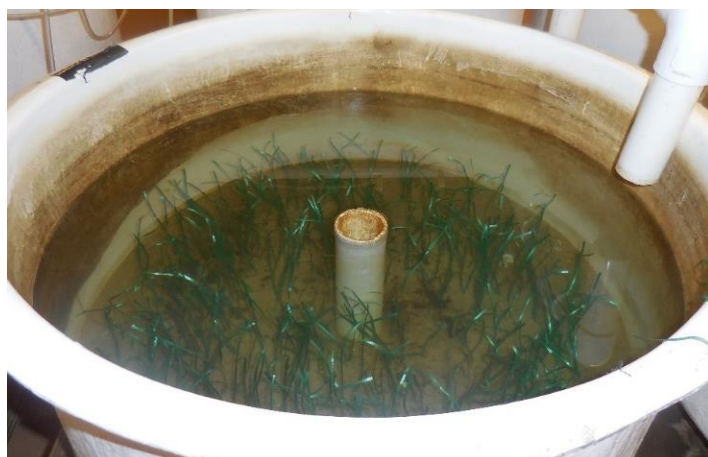
Figure 8. Two circular tanks contained simulated Ruppia maritima meshes weighted with rebar and covered with 1-5 cm of sand. The green polypropylene ribbons attached to the meshes were pulled up from underneath the sand.
