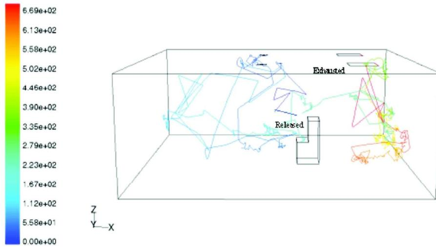
Particle tracking prediction from the computational fluid dynamics model for the 6 ACH summertime condition. Only one tracked particle is shown in the figure. The color legend is the residence time in seconds of the particle released.
