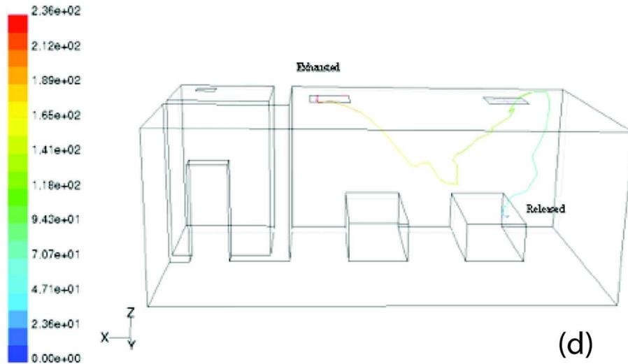
CFD particle tracking in three hospital rooms: (a) patient room with upper-room UVGI and particle released from middle of the room, (b) patient room with upper-room UVGI and particle released from bed, (c) exam room with upper-room UVGI with particle released at exam bed, and (d) patient room with ducted UVGI system and particle released from a bed. The color legend is the residence time in seconds of each particle released.
