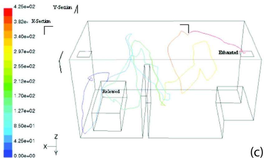
CFD particle tracking in three hospital rooms: (a) patient room with upper-room UVGI and particle released from middle of the room, (b) patient room with upper-room UVGI and particle released from bed, (c) exam room with upper-room UVGI with particle released at exam bed, and (d) patient room with ducted UVGI system and particle released from a bed. The color legend is the residence time in seconds of each particle released.
