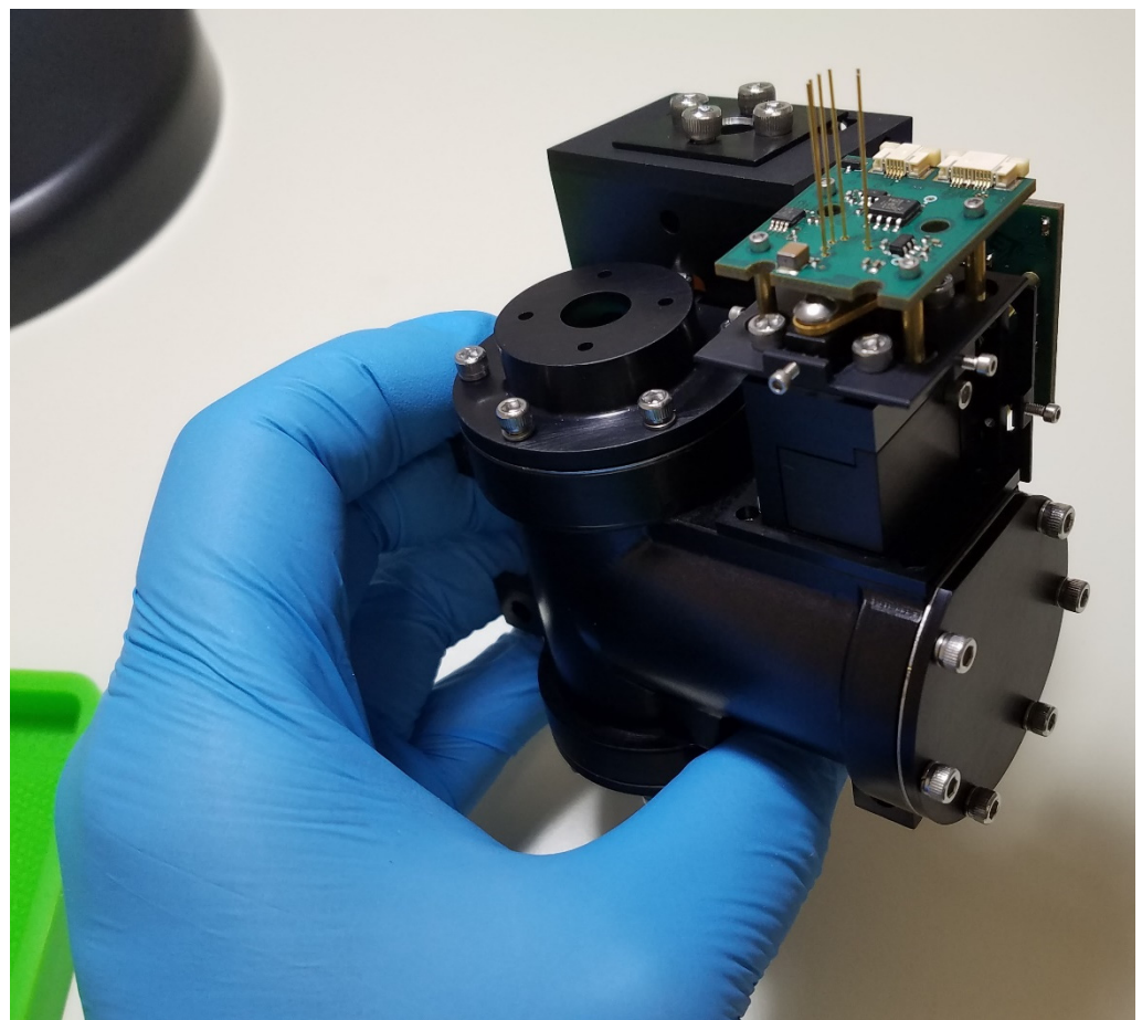
Figure 8. In this photo, the AFN is at 80% completed assembly. Here, is shown the entire optical assembly with detector electronics.
