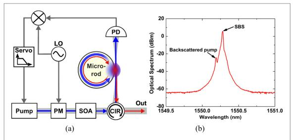
**Figure 1.** SBS microrod laser. (a) Configuration of the SBS laser that employs a commercial integrated planar external-cavity diode laser to pump a high-Q microrod cavity. (b) The output optical spectrum of the SBS laser exhibiting 3.7 mW power at 1550 nm wavelength.
