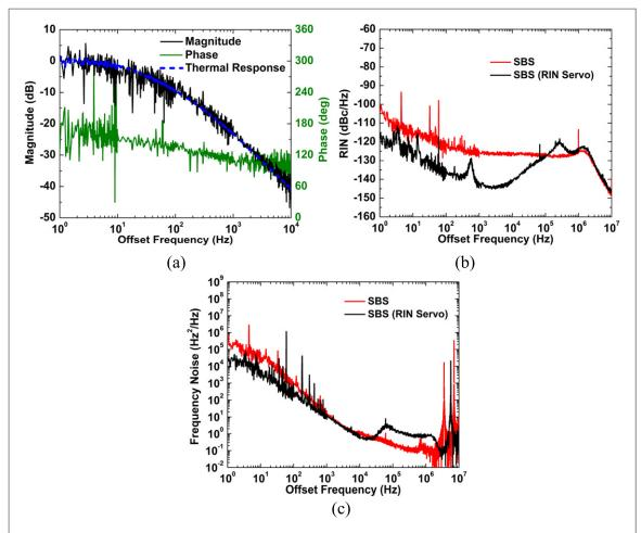
Figure 5. SBS microrod laser noise feedback. (a) Frequency response between SBS RIN and SBS frequency noise indicating a rolloff that matches the microrod thermal response. (b) RIN of the SBS laser showing 10–20 dB noise improvement upon servo control of the SBS intensity fluctuations. (c) SBS laser frequency noise showing an improvement at low offset frequencies as a result of the RIN servo.
