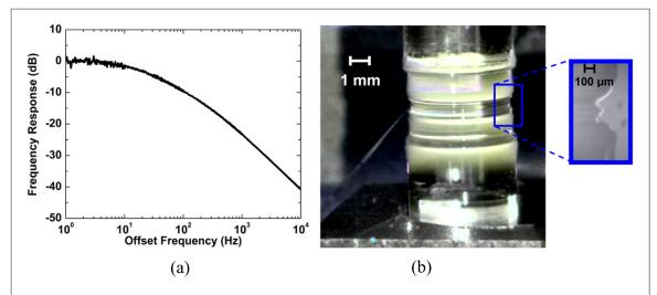
**Figure 3.** Thermal properties of the SBS microresonator. (a) Thermal response of the SBS microred indicating a 3 dB bandwidth of 18 Hz. (b) Photograph of the SBS microred resonator having a fabricated resonator minor diameter of 170  $\mu$ m.
