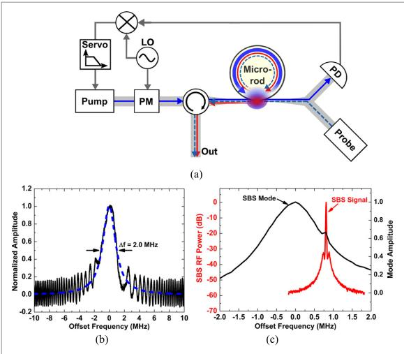
**Figure 2.** Measurement of the SBS laser operating parameters. (a) Configuration of the measurement setup used to determine the loaded *Q* of the microrod. (b) Profile of the pump mode illustrating zero cavity detuning and also a 2.0 MHz Lorentzian width. (c) Profile of the SBS mode illustrating a SBS detuning of 810 kHz.
