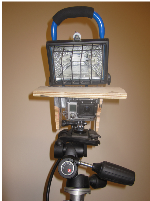
Figure 3.12: The camera setup featuring the GoPro, with its protective glass casing and wooden heat insulator, and the floodlight.
