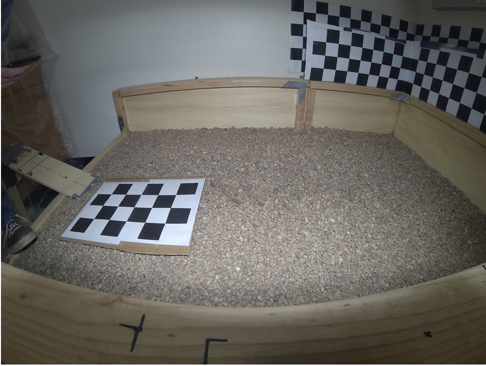
Figure 3.16: The calibration pattern (chessboards) on the wall are used to compute the direction of the x , y and z axes of the box frame.
