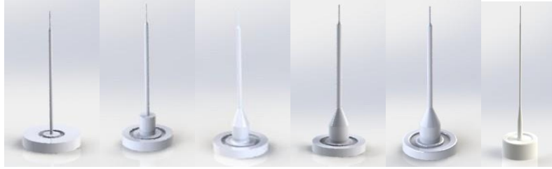
Figure 7.7: CAD renderings of the geometry of the mandrel highlighting the changing geometry with the evolution of process capabilities (left: oldest, right: newest)
