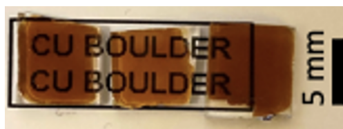
Figure 3.3: Optical image of three nanocomposite films with different Tb 3+ doping densities of 0.29 % (left), 1.12 % (middle), and 4.55 % (right). The optical clarity is demonstrated by the clearly visible letters behind the film that do not exhibit any scattering.
