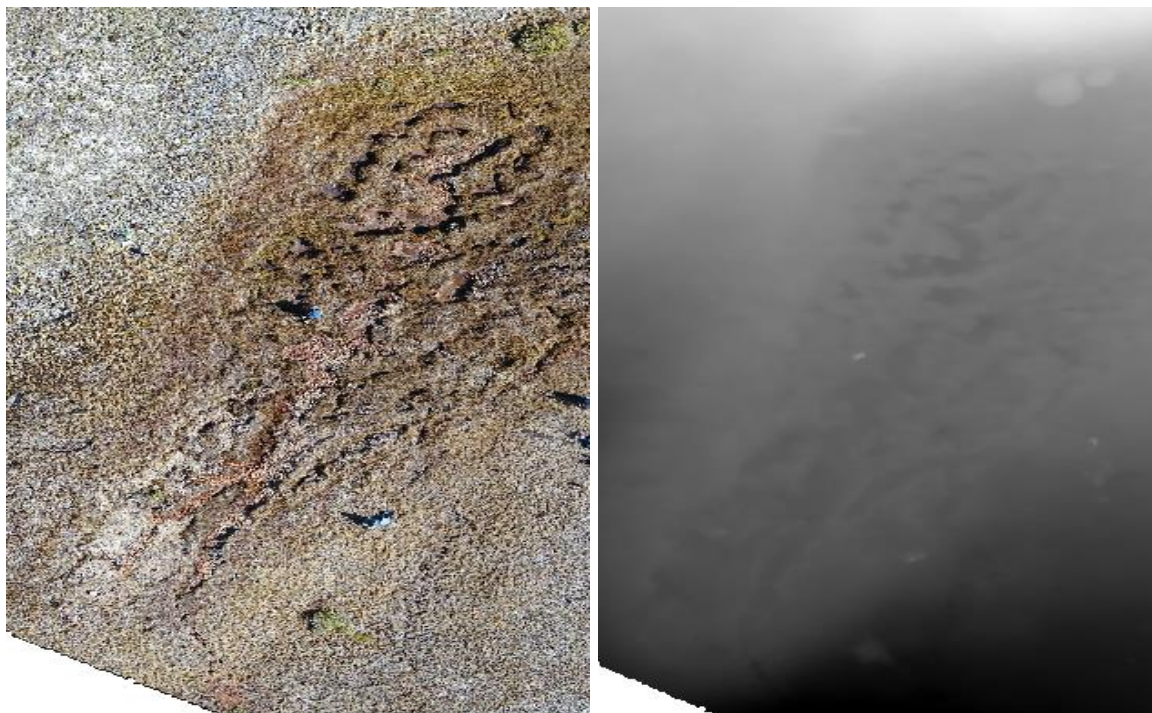
Figure 4: .tif image (left) and DSM (right) of Lobe 45 taken by the Phantom 4 on 9/22/17 and compiled using Maps Made Easy software. Lighter color on the DSM indicates higher values for elevation.
