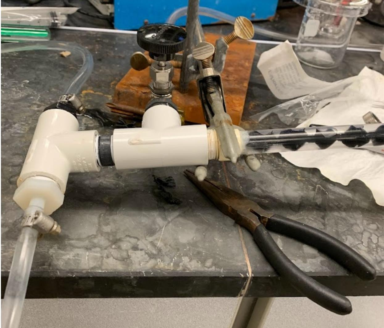
**Figure 7:** Initial static mixer inflow setup for 0.5" diameter mixer.
