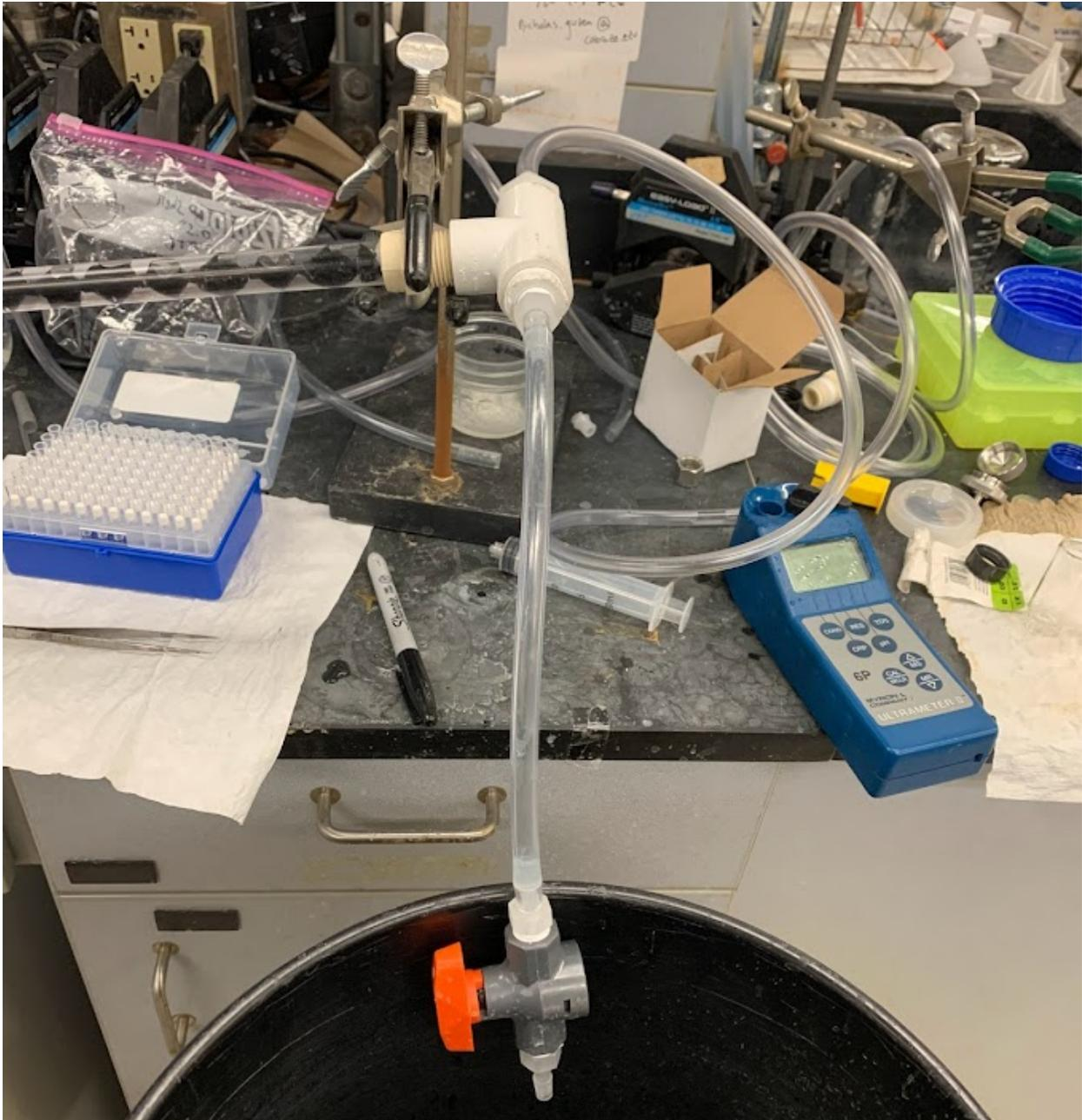
**Figure 8:** Static mixer outflow setup for 0.5" diameter tubing.
