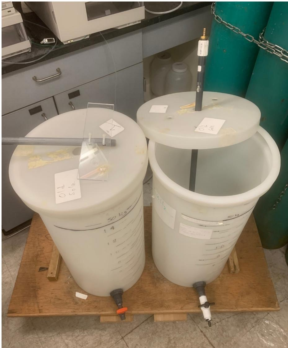
**Figure 5:** The two 50 L tubs with stir sticks used for all experiments, unless noted otherwise.
