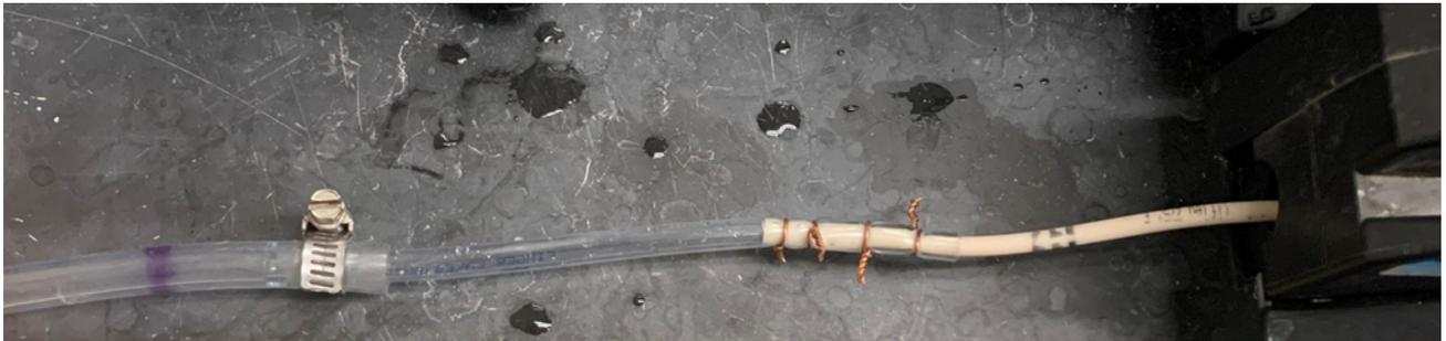
*Figure 6: The tubing set up including the intermediate tubing to bridge the size gap.*
