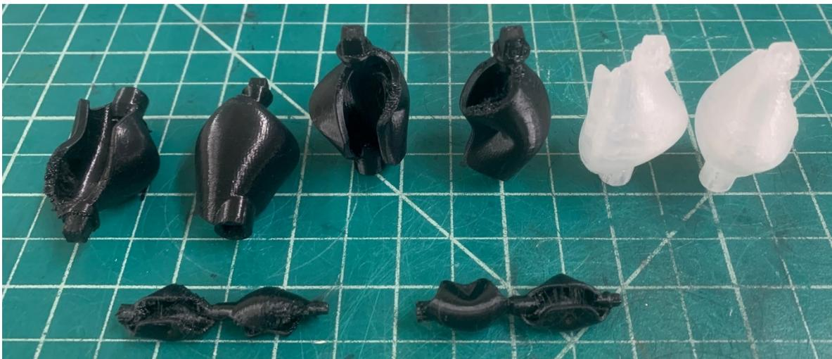
**Figure 3:** Shell static mixer inserts at 1" and 1/2" diameters.
