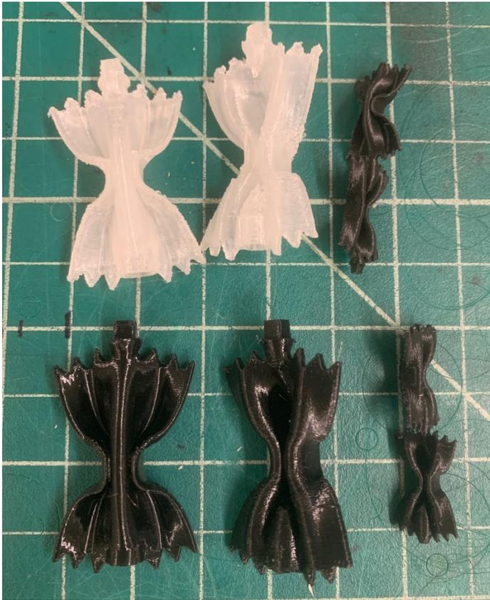
*Figure 1: Farfalle static mixer inserts at 1" and 1/2" diameters.*
