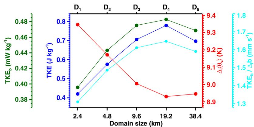
**Figure 7.** Boundary layer production of turbulence kinetic energy due to buoyancy  $TKE_b$ , boundary layer TKE, jump in virtual potential temperature across the inversion  $\Delta_l(\theta_v)$ , and entrainment parameter  $TKE_b / \Delta_l b$  (equation (2)), day 8–10.
