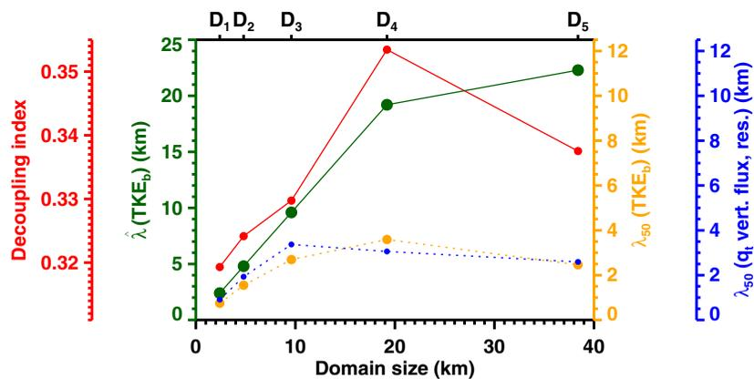
**Figure 4.** Decoupling index and cell scale ( $\hat{\lambda}$ ) of buoyant TKE production in the boundary layer, and median scale ( $\lambda_{50}$ ) of buoyant TKE production in the boundary layer and of the vertical resolved-scale flux of total water at mean cloud base, day 8–10.
