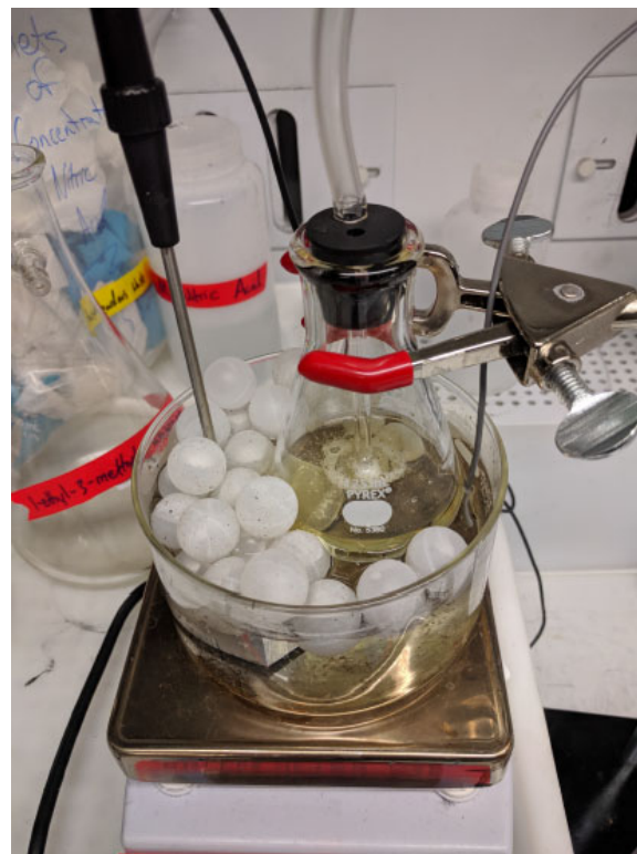
Fig. 6. Assembly for sparge desorption of CO 2 from [bmim][Ac].
