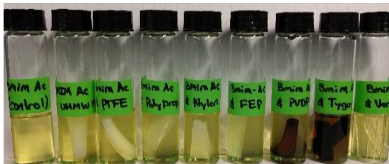
Fig. 7. Material compatibility samples compared to a control; 23^\circ\text{C} \pm 1^\circ\text{C} .
