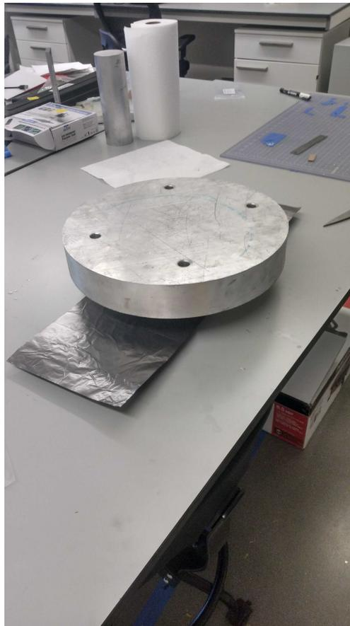
Figure 2.12: Image of a 16 kg weight on top of the press jig used to attach layers to the bracket
