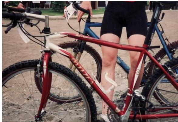
**Fig 1: Buckled bicycle frame. Source:**
