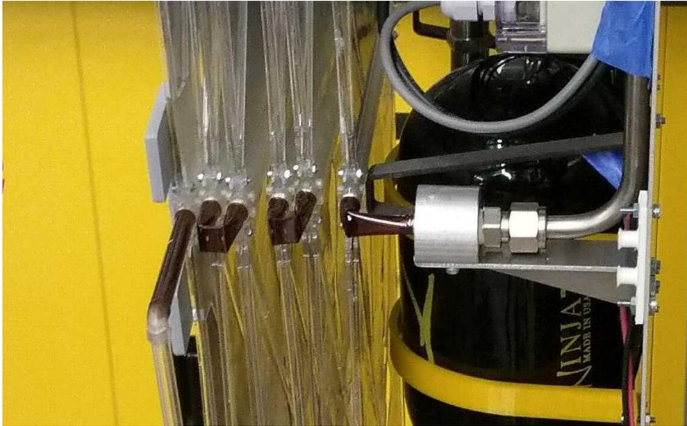
Figure 2.19: Close up view of thin kinked polyimide tubes connecting panels together in a prototype
