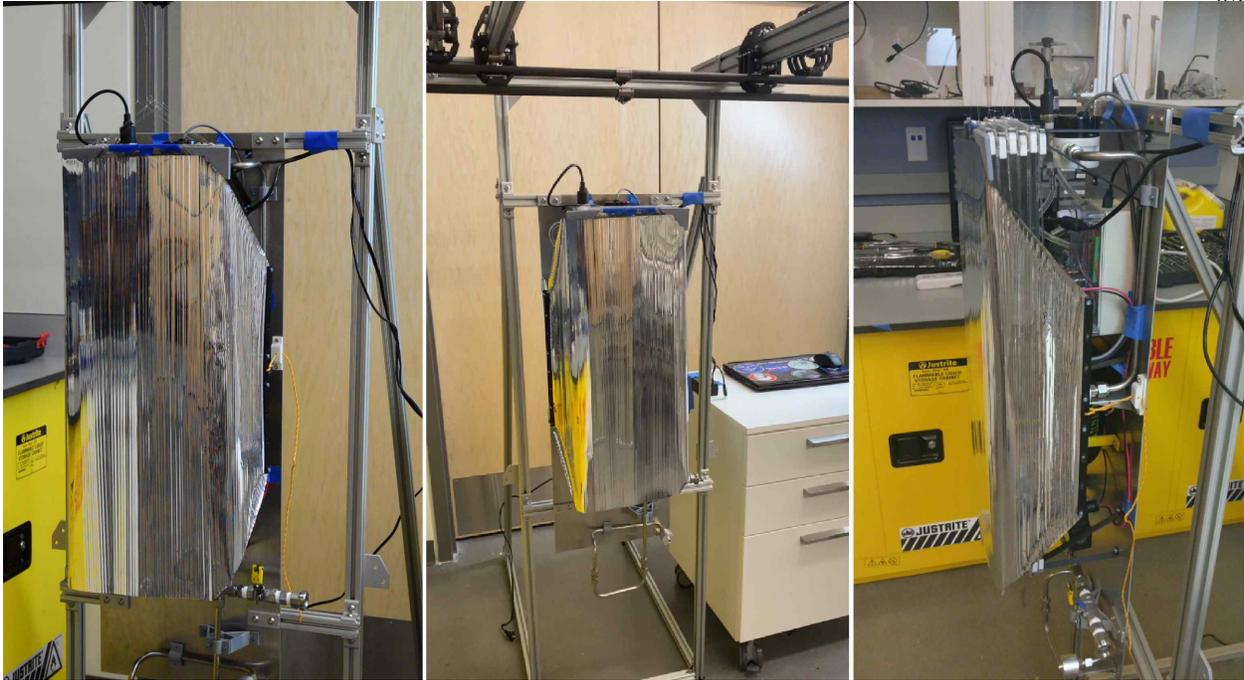
Figure 4.28: Left: packaged deployment prototype front view. Center: Packaged deployment prototype with staggered sliding rails. Right: Packaged deployment prototype side view
