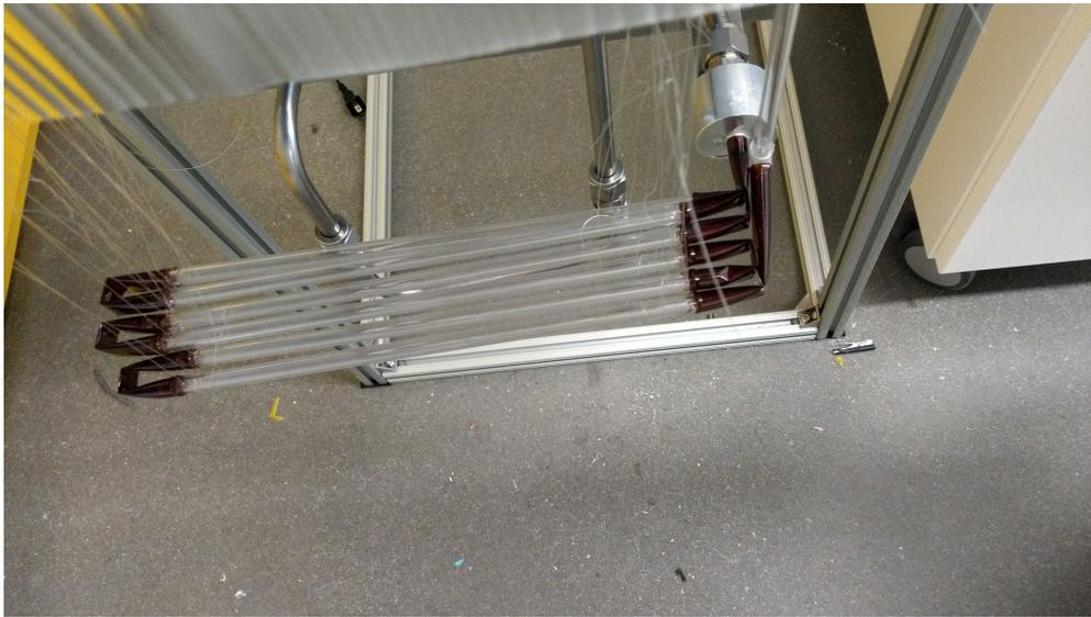
Figure 4.25: Image of the lower tubes representing what would be a second set of panels in the proposed design. They are hung using strings attached to the panels above
