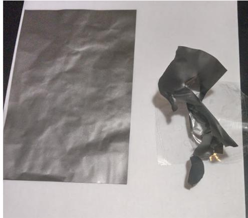
Figure 2.10: PGS without adhesive backing that ripped immediately after pulling it out of its package
