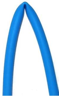
**Fig 5: Kinked Hose - an example of a tube in the post-buckling state. Source: Kyle Marquis**
