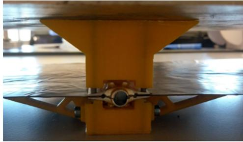
Figure 2.13: Image of the press jig clamping two shells of the clamping tube bracket around PGS layers
