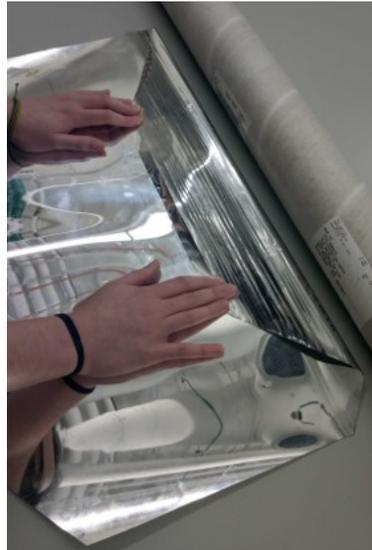
Figure 4.27: Rolling the PET film by hand
