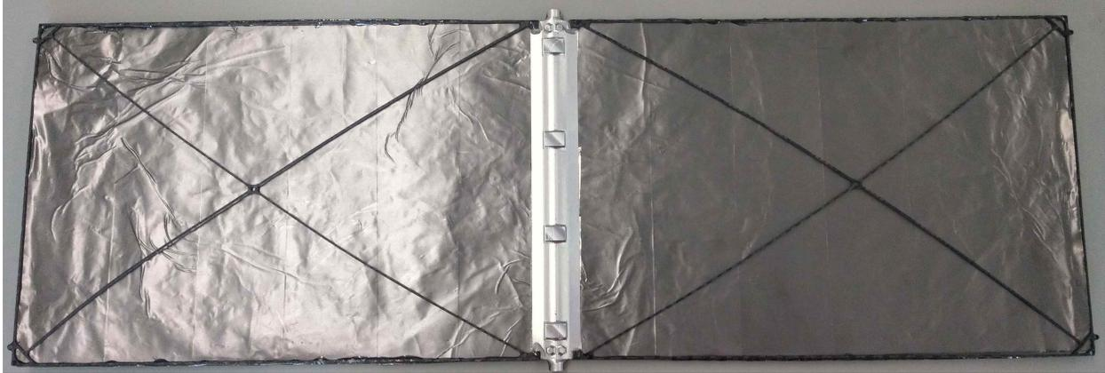
Figure 2.8: Top view of the radiator panel prototype
