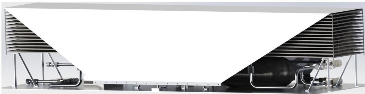
Figure 2.14: Packaged view of the proposed deployable radiator system held down via scroll sheet
