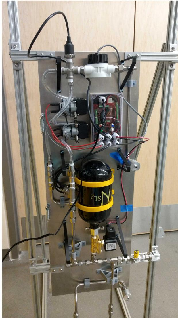
Figure 4.24: Image of the prototype fluid loop system without the radiator panels attached. Pictured here is an accumulator, pressure sensors, a solenoid valve, a flow sensor, check valves, pumps, the tubing, and the electronics for control and measurement
