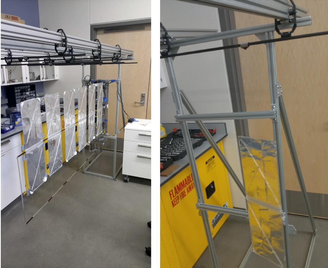
Figure 4.23: Left: two-axis gravity compensation rail system built and operational. Right: video demonstration of two-axis motion for a single panel being pulled along. [Link](#)
