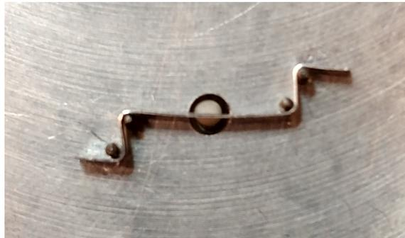
Figure 3.10: A view of the strip in the bending jig. The Torr Seal ball lines up with the hole in the center.
