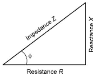
Figure 3-3 Relationship between resistance, impedance, and reactance. [44]
