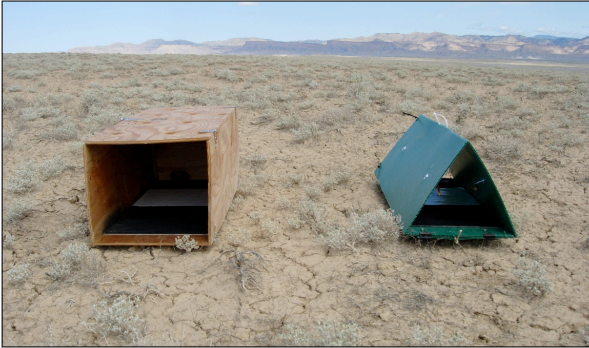
Figure 3. Kit fox detection stations. Track-plate box (left). Two-in-one hair snare/track-plate detection station (right).
