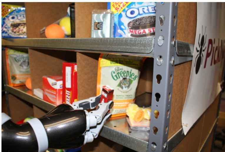
Figure 1.1: A storage shelf from an Amazon warehouse with a Kinova Jaco 2 arm reaching into a confined space for products used in the Amazon Picking Challenge [37]
