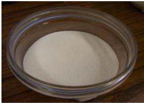
a) PCM powder at room conditions [264]
