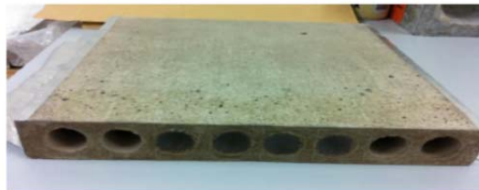
c) PCM-enhanced hollow core floor
