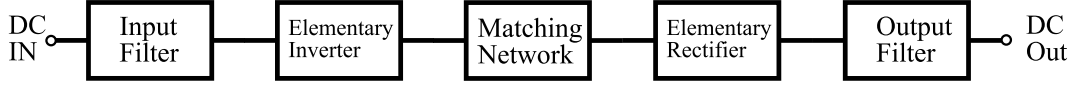
Figure 3.1: Diagram of the synthesis of dc-dc converters by cascading fundamental two-port networks
