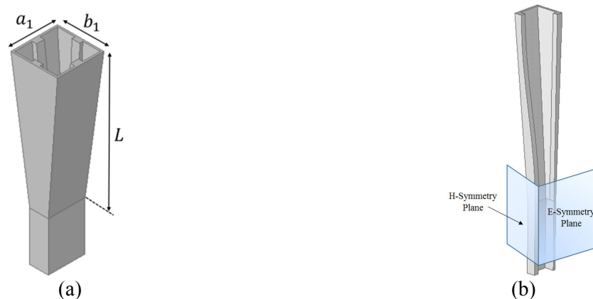
Figure 4.14. (a) Prototype horn 2 full model and (b) defined using E and H symmetry planes.
