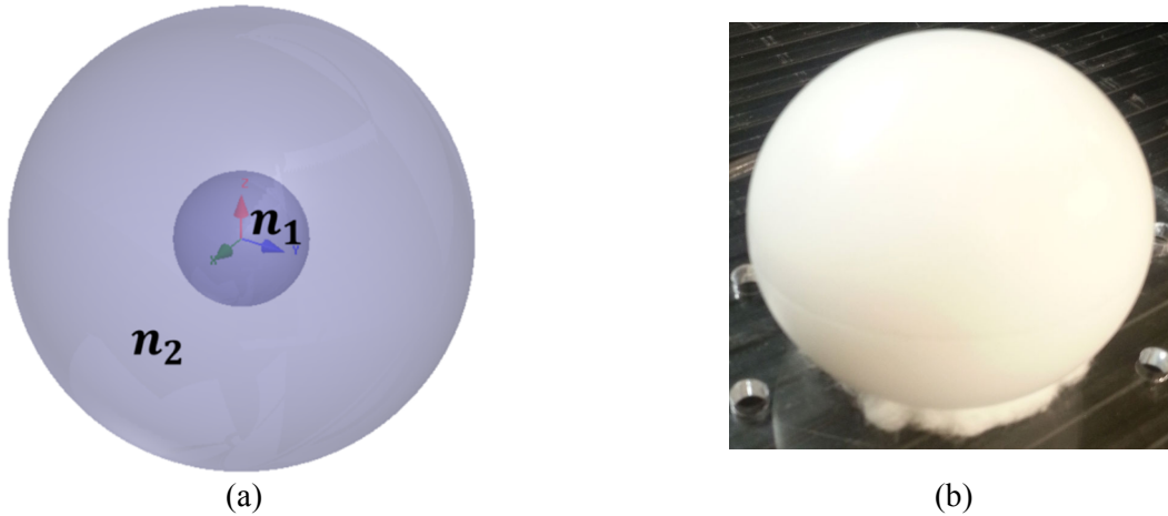
Figure 5.1. (a) 2-layer LL HFSS model with transparent outer layer and (b) manufactured lens.
