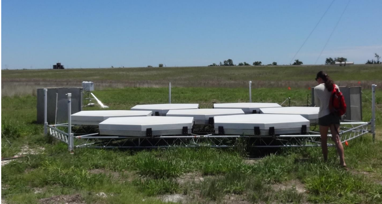
Figure 1.5. 449 MHz radar wind profiler as set at NCAR FP3, June 2015
