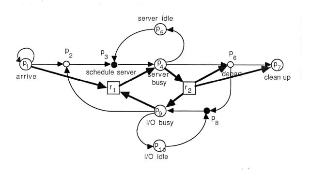
Figure 3: A Pictorial Representation of the BPG in Figure 1
