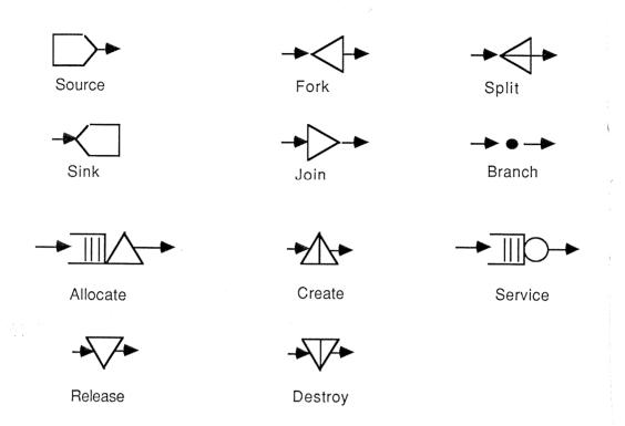
Figure 5: Extended Queueing Network Nodes
