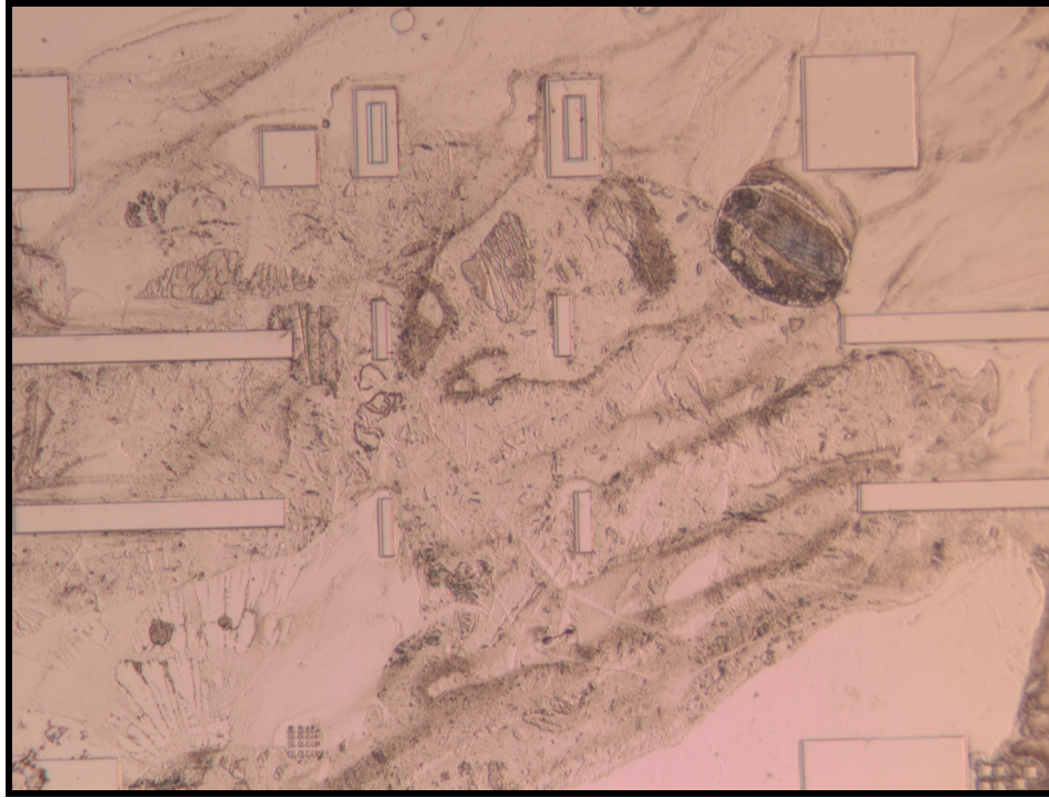
Figure 4.3: Micrograph of failed GaAsBi RIE using a \text{BCl}_3 etch gas
