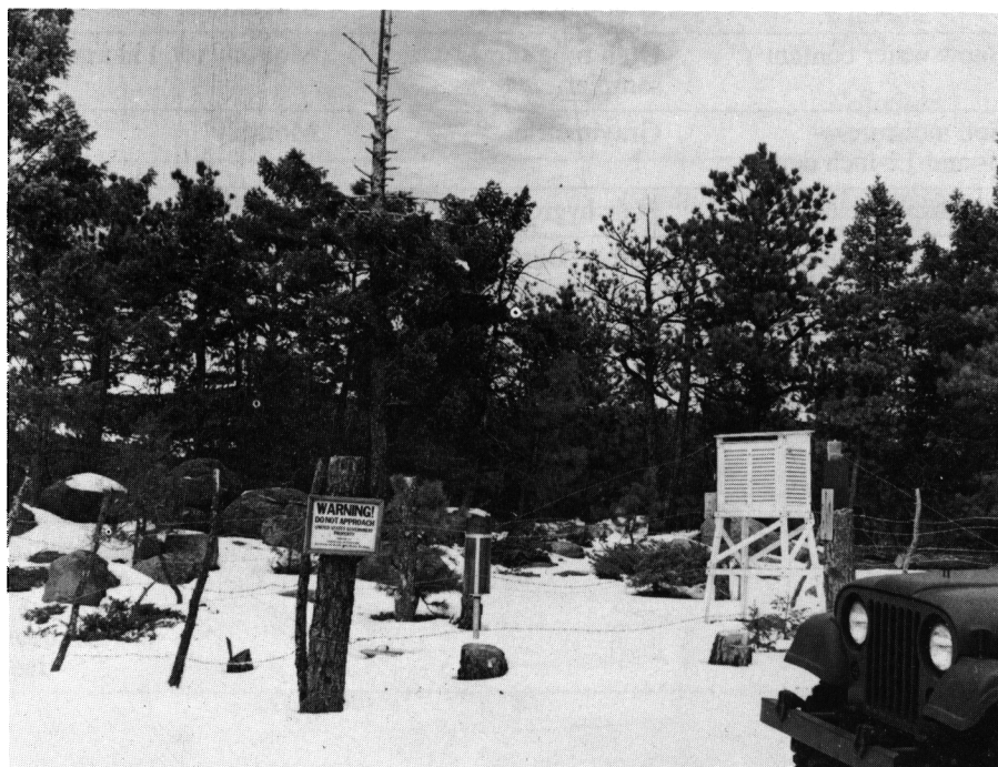
FIGURE 2. The Lower Montane (A-1) station at 7,200 feet elevation. The anemometer is mounted in the top of the tree with branch stubs in the left background.
