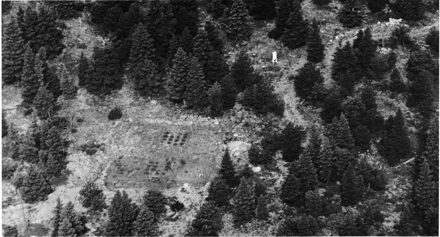
FIGURE 3. Aerial view of the Upper Montane (B-1) station at 8,500 feet elevation. The anemometer was mounted at the top of the dead tree with boulders at its base to the right of the white instrument shelter. The pattern of squares in the lower left portion of the photograph is a transplant garden. National Center for Atmospheric Research photograph.
