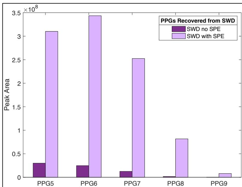
**Figure 4.4: Peak area of PPGs with and without SPE in SWD.**
