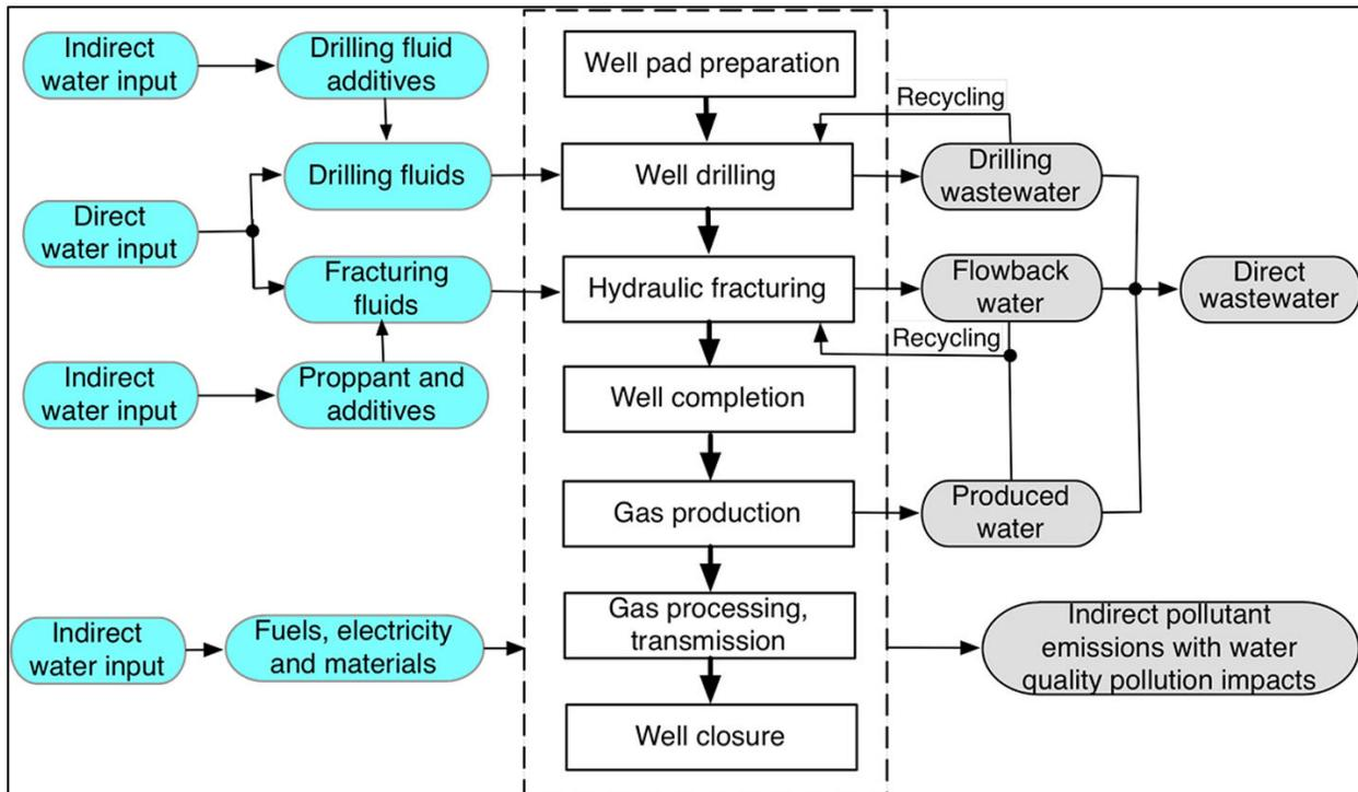
Figure 1.3: Water cycle for hydraulic fracturing [43].
