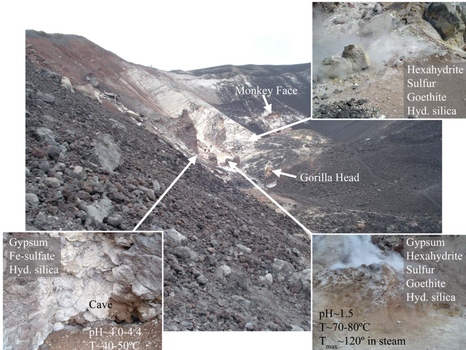
Figure 7. Field images of Cerro Negro with mineralogy identified by in situ VNIR reflectance spectroscopy and environmental parameters.
