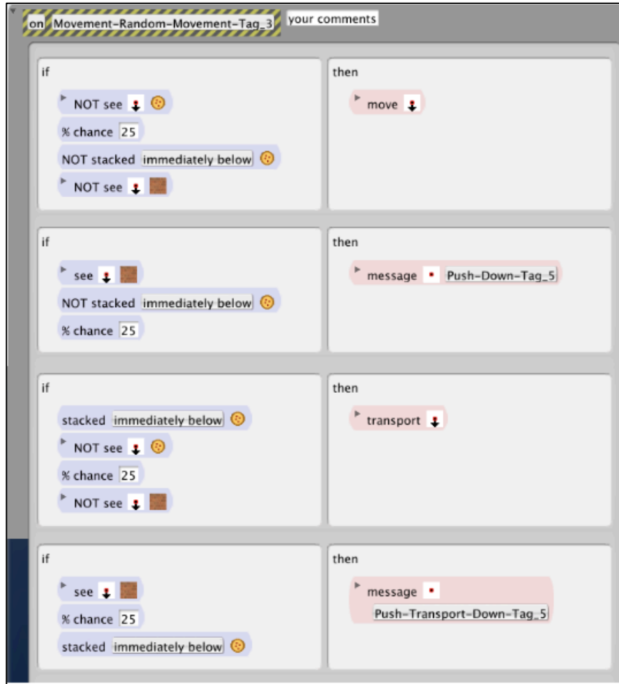
Figure 53: The Move Down Rule In The Random Movement Method With The Push And Transport Modulating Patterns Applied
