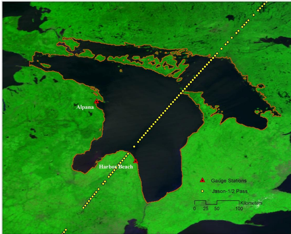
Figure 5.3 The exact ground tracks of Jason-1 and Jason-2 descending orbit overpassing Lake Huron
