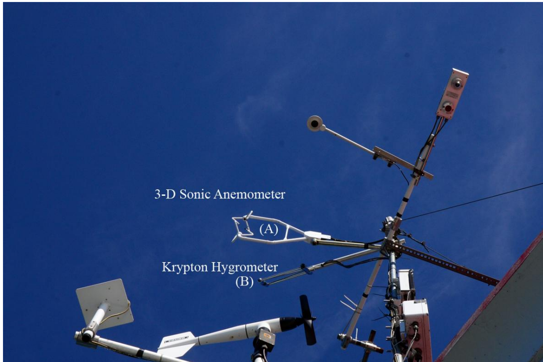
Figure 4.1 3-D sonic anemometer (A) and Krypton Hygrometer (B) located on the roof of Spectacle Reef Lighthouse. These are the major instruments providing meteorological and flux data for calculating and validating latent and sensible heat fluxes, September, 2014. Credit: Pakorn Petchprayoon
