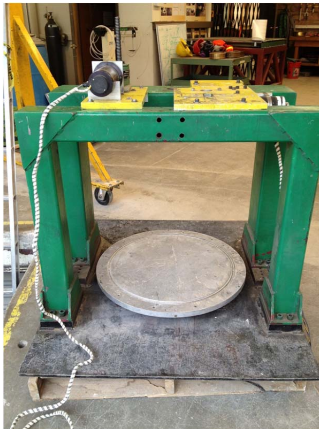
Figure 3.10: Loading frame for the 400 g-ton geotechnical centrifuge
