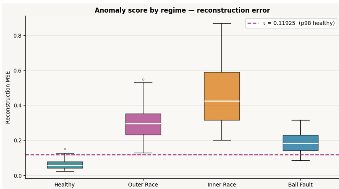
Figure 6: Residual distributions produced by the learned representation operator. The operator is trained only on nominal trajectories. The separation between nominal and non-nominal regimes indicates that the learned residual is diagnostically meaningful as a proxy for distance to the nominal quotient manifold.
