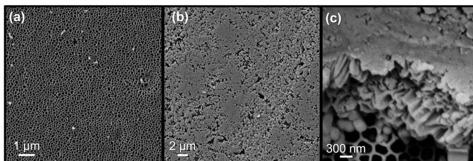
**Figure 8.** (a) SEM image of the pristine AAO surface in the absence of 9MA and polishing. (b) At low magnification, SEM image of the polished surface of a 9MA-filled template. (c) High magnification SEM image of the polished surface of a 9MA-filled template, showing surface debris that covers the channels and has been smoothed by polishing.
