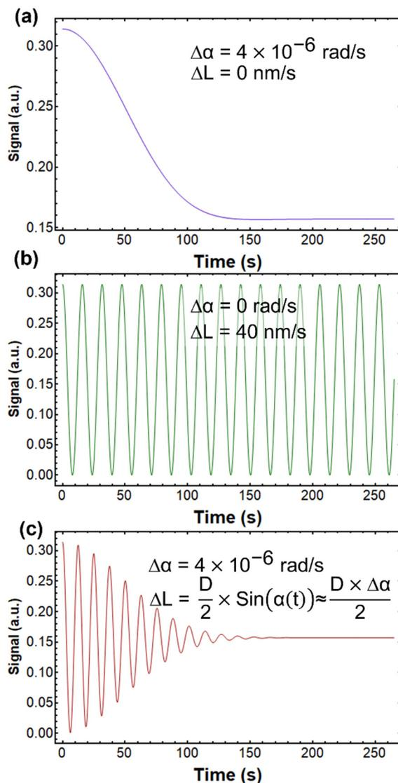
**Figure 6.** Simulated interferograms generated using Equation (2) with the parameters listed in the figures. Patterns caused by changes in either (a) the angular error or (b) the optical path difference do not agree with the data in Figure 5. Only when (c) both parameters change is an interferogram that is comparable to that in Figure 5 obtained.  $\Delta L$  and  $\Delta\alpha$  are as described in the main text and  $D$  is the diameter of the AAO template.
