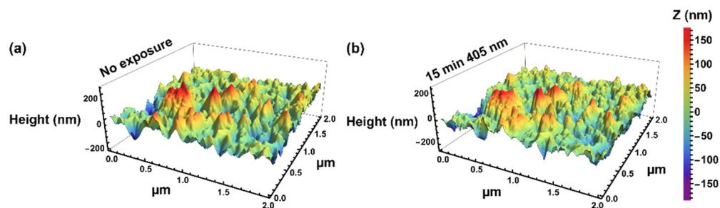
**Figure 7.** Atomic force microscope scan of a 9MA-filled template irradiated in-situ with a diffuse 405 nm laser. (a) before the 9MA was photo-dimerized and (b) after 15 min of exposure to 405 nm. There are slight changes in individual features but no obvious protrusions of nanowires from the surface.
