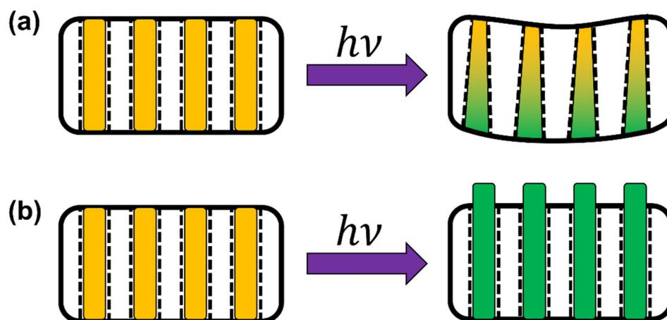
**Figure 1.** Schematic representation of the two possible methods of actuation in the organic-template system, (a) partial reaction of the crystal causing a change in curvature of the template and (b) full reaction of the crystal causing extension of organic nanorods through the surface of the template.
