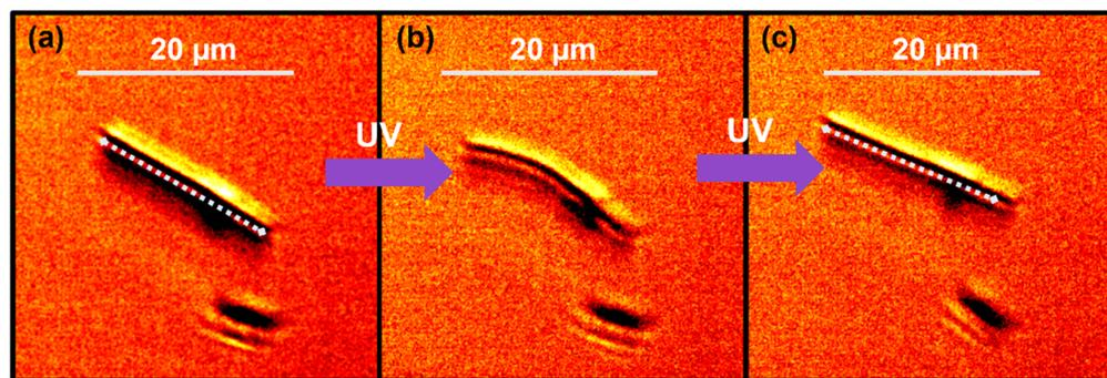
**Figure 4.** Optical microscope images of a **9MA** nanorod suspended in aqueous solution (a) before, (b) during, and (c) after exposure to UV light. The nanorod extends roughly 7% along its long axis.
