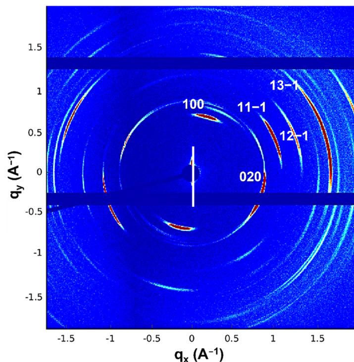
**Figure 3.** The GIWAXS pattern and accompanying face indexation for a  $3\text{ mm} \times 1\text{ mm}$  sample cut from a **9MA**-filled template. The film plane direction is indicated by the white line near the origin. The FWHM of the scattering is  $3.7^\circ$  in the azimuthal direction, indicating that the sample is highly oriented along the film normal and thus inside the pore axis.
