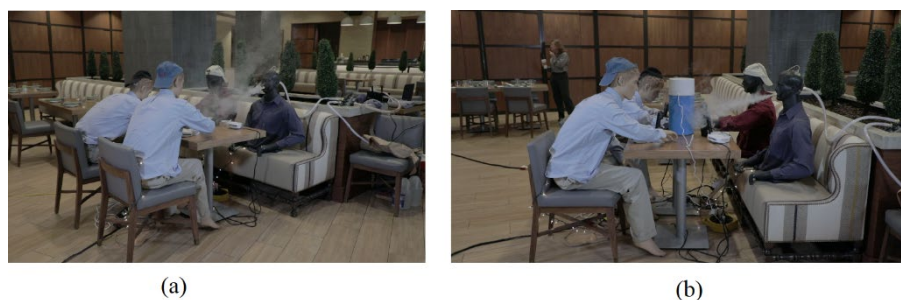
Figure 14. The dispersion processes of stage fog (a) without and (b) with purifier in a restaurant.
