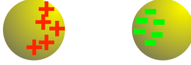
Figure 3.2: Graphical interpretation of uneven charge distribution on spheres in close proximity
