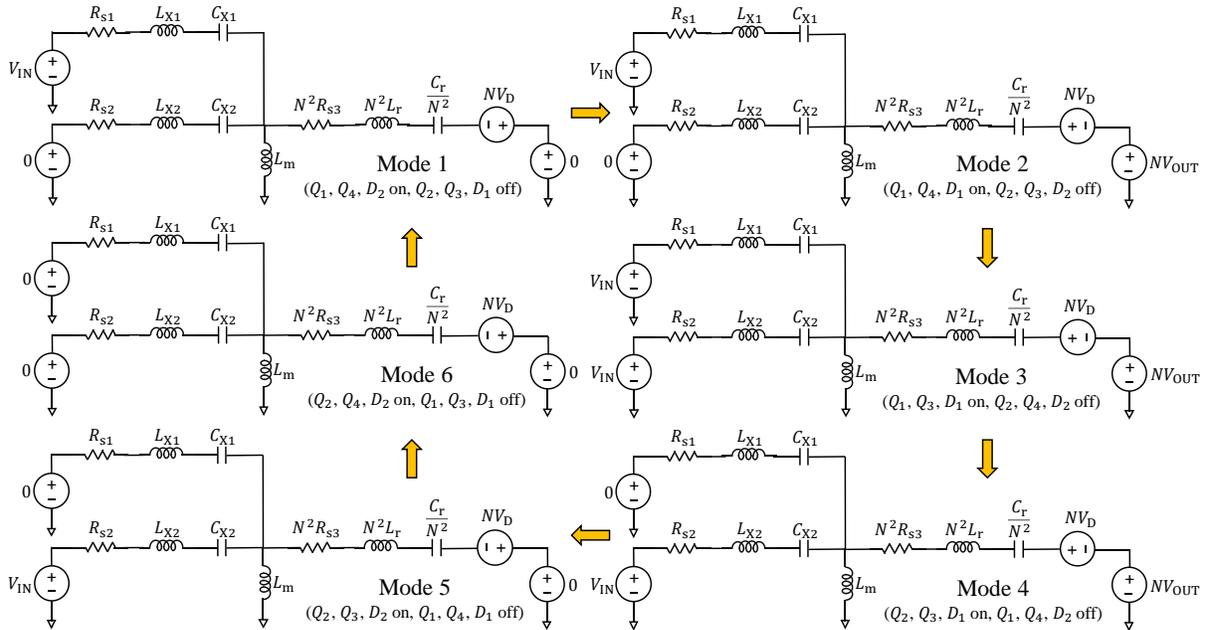
**Figure 2.6:** The six linear operating modes of the impedance control network (ICN) converter of [23].
