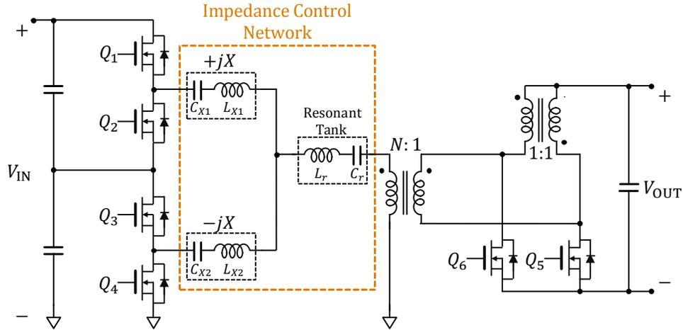
**Figure 6.2:** ICN resonant converter with stacked inverters and a resonant current-doubler rectifier.
