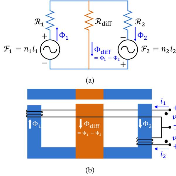
**Figure 4.5:** Proposed approach for realization of the integrated magnetic structure: (a) magnetic circuit, and (b) implementation. The primary flux paths are shown in blue, and the differential flux path is shown in orange.
