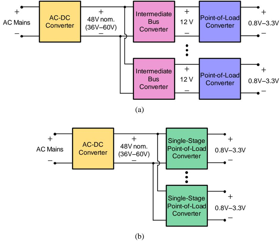
**Figure 1.3:** Datacenter power distribution architectures: (a) conventional architecture with three power conversion stages in each path from source to load, and (b) modern architecture with one power conversion stage eliminated by replacing intermediate bus converters and point-of-load converters by single-stage point-of-load converters.
