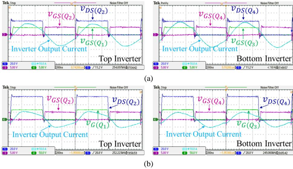
**Figure 3.8:** Measured waveforms confirming ZVS and near-ZCS operation of the inverters of the ICN resonant converter operating at full power (390 W) at: (a) 36 V input voltage and 34 V output voltage, and (b) 60 V input voltage and 34 V output voltage. Waveforms shown are the output voltage, output current, and gate signals of the two half-bridge inverters.
