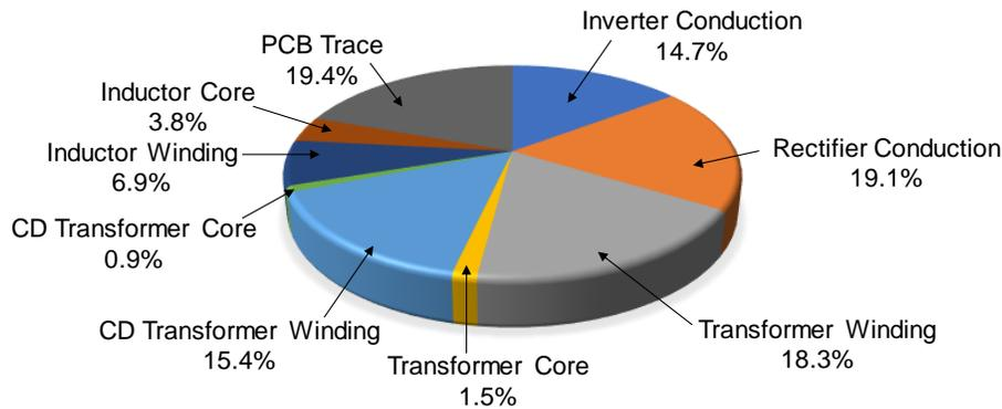
**Figure 6.10:** Theoretically predicted loss breakdown of the first PoL ICN converter prototype, operating at  $V_{IN} = 36 \text{ V}$ ,  $V_{OUT} = 1.8 \text{ V}$  and  $P_{OUT} = 90 \text{ W}$ . Here, “IN” is an abbreviation for immittance network, and “CD” is an abbreviation for current-doubler.
