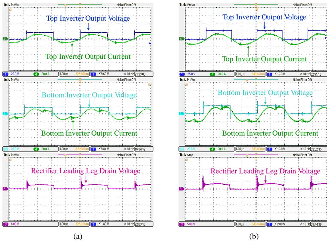
**Figure 6.8:** Inverter and rectifier switching waveforms of the first PoL ICN converter prototype while delivering 90-W output power at: (a)  $V_{IN} = 36$  V and  $V_{OUT} = 1.8$  V, and (b)  $V_{IN} = 48$  V and  $V_{OUT} = 1.8$  V.
