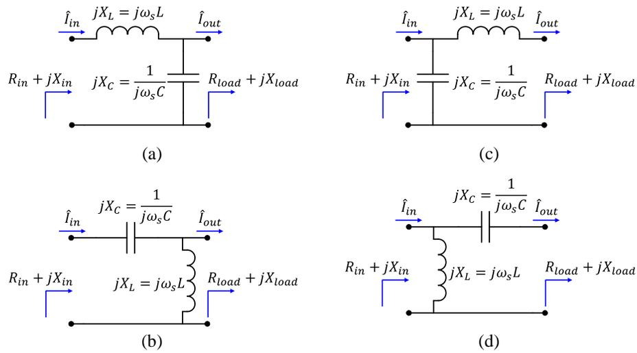
**Figure 8.1:** Four different types of L-section stages. Under the conventional design approach, the input and load reactances ( $X_{in}$  and  $X_{load}$ ) of all such stages in a multistage matching network are constrained to be zero, while the proposed approach allows  $X_{in}$  and  $X_{load}$  to have non-zero values.
