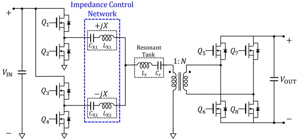
**Figure 5.1:** Impedance control network (ICN) dc-dc converter with a full-bridge synchronous rectifier.
