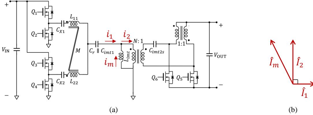
**Figure 7.1:** Reason behind relatively large core losses in the immittance network transformer of the second PoL ICN converter: (a) converter topology illustrating the input, output and shunt-branch (magnetizing) currents of the immittance network transformer, and (b) phasor representation of these currents.
