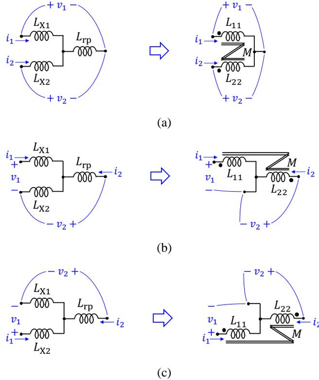
**Figure 4.3:** Realization of the three inductors of the ICN converter using two coupled windings in three topologically distinct ways. In (a),  $L_{X1} = L_{11} - M$ ,  $L_{X2} = L_{22} - M$  and  $L_{rp} = M$ ; in (b),  $L_{X1} = L_{11} - M$ ,  $L_{X2} = M$  and  $L_{rp} = L_{22} - M$ ; and in (c),  $L_{X1} = M$ ,  $L_{X2} = L_{11} - M$  and  $L_{rp} = L_{22} - M$ .
