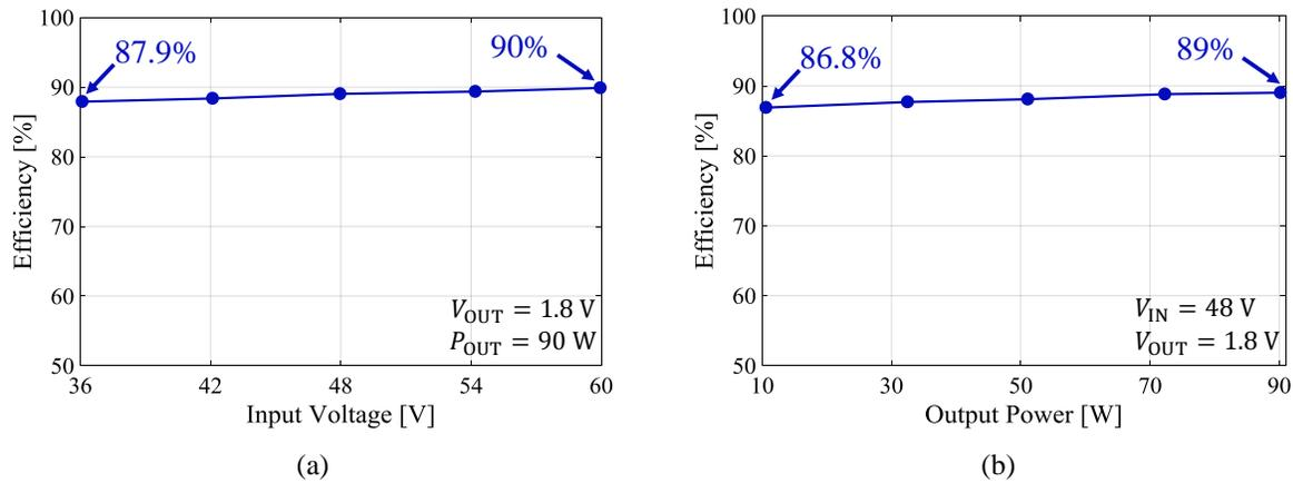
**Figure 6.21:** Measured efficiency of the second PoL ICN converter prototype: (a) as a function of its input voltage at full power ( $P_{OUT} = 90\text{ W}$ ), and (b) as a function of its output power at its nominal input voltage ( $V_{IN} = 48\text{ V}$ ). In both (a) and (b), the output voltage  $V_{OUT} = 1.8\text{ V}$ .
