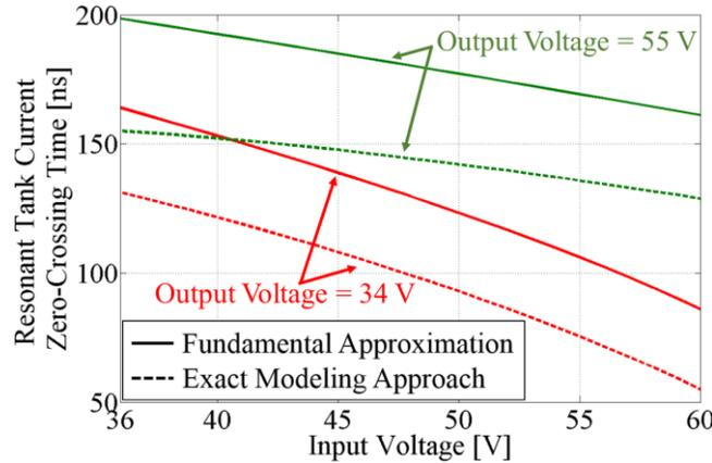
**Figure 3.5:** Zero-crossing time of resonant tank current (with respect to switching-time of top inverter), as predicted by the fundamental approximation (solid lines), and by the exact modeling technique (dashed lines), for an output voltage of 55 V (green) and 34 V (red).
