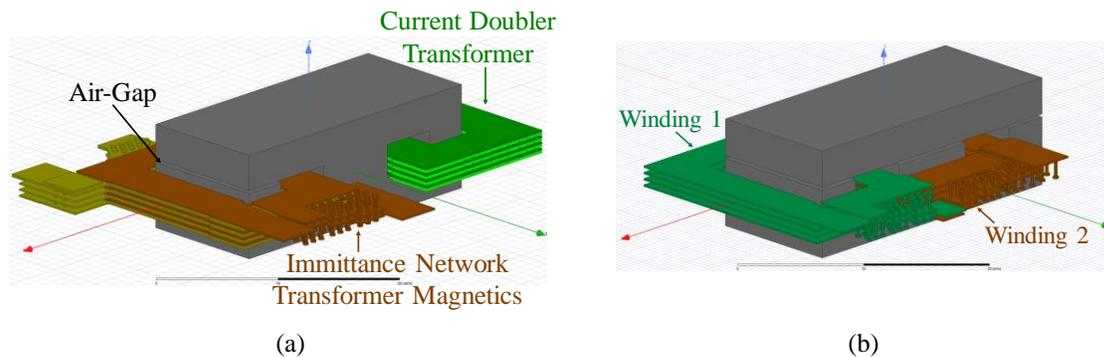
**Figure 6.18:** Maxwell 3D models of the two integrated magnetic structures of the PoL ICN converter of Fig. 6.16: (a) immittance network and current-doubler transformers, (b) ICN inductors.
