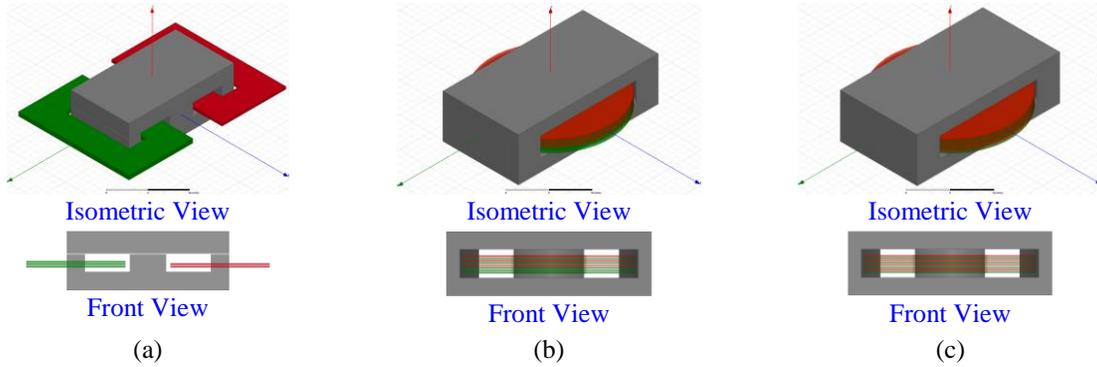
**Figure 6.5:** Models of the three magnetic components of the PoL ICN converter of Fig. 6.4 implemented in Maxwell 3D: (a) integrated magnetic structure, (b) main transformer, and (c) 1:1 resonant current-doubler transformer.
