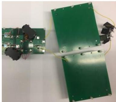
**Figure 9.6:** Photograph of the prototype capacitive WPT system incorporating a variable compensation inverter.
