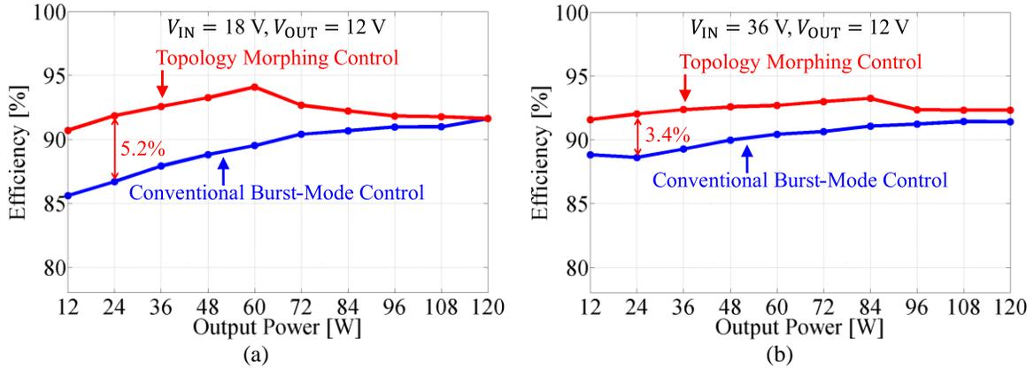
**Figure 5.19:** Measured efficiency of the ICN converter under topology morphing control and conventional burst-mode control across variations in output power at: (a) input voltage of 18 V, and (b) input voltage of 36 V.
