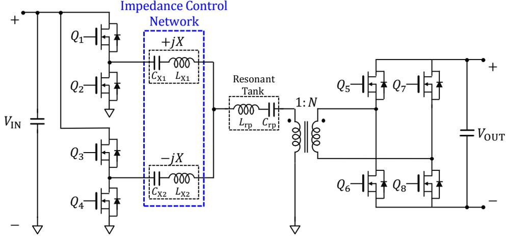
**Figure 4.1:** Impedance control network (ICN) resonant dc-dc converter with its three inductors connected at a common node, forming a T- network.
