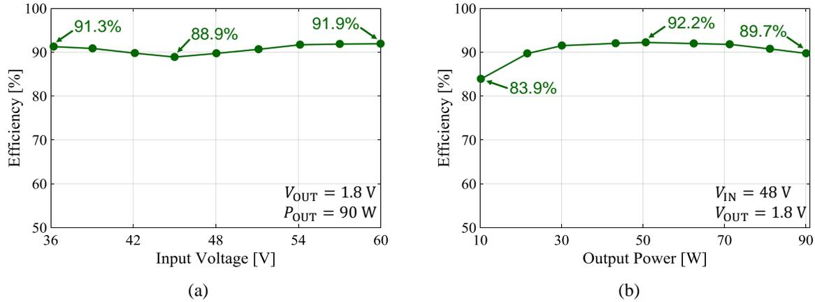
**Figure 7.11:** Measured efficiency of the final PoL ICN converter prototype: (a) as a function of its input voltage at full power ( $P_{OUT} = 90\text{ W}$ ), and (b) as a function of its output power at its nominal input voltage ( $V_{IN} = 48\text{ V}$ ). In both (a) and (b), the output voltage  $V_{OUT} = 1.8\text{ V}$ .
