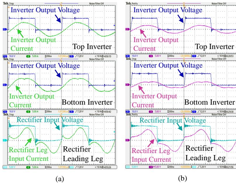
**Figure 5.16:** Steady-state switching waveforms of the ICN converter when operating at  $V_{IN} = 18$  V and  $V_{OUT} = 12$  V with the rectifier operating in (a) full-bridge mode, and (b) half-bridge mode.
