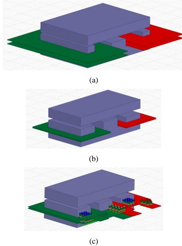
**Figure 4.7:** 3D finite element analysis based design optimization of the integrated magnetic structure: (a) initial core and winding geometry, (b) optimized geometry and (c) optimized geometry as implemented in a printed circuit board, including vias and winding terminals.
