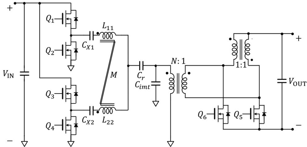
**Figure 7.4:** ICN converter with the inductances of its immittance network realized using the coupling of the ICN inductances and the leakage inductance of the transformer.
