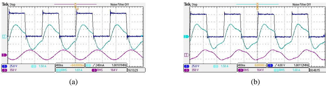
**Figure 8.9:** The inverter output voltage, matching network input current (top waveforms, in blue) and load voltage (bottom waveforms, in pink) for the two matching network designs operating at an output power of 100 W: (a) conventional approach and (b) proposed approach.
