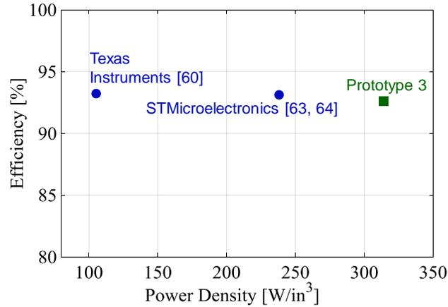
**Figure 7.13:** Performance comparison of the final PoL ICN converter prototype with state-of-the-art single-stage isolated 48V-to-1.8V point-of-load converters. For the efficiency comparison, the peak efficiency of each converter is considered. For the power density comparison, only the power stage of each converter is considered.
