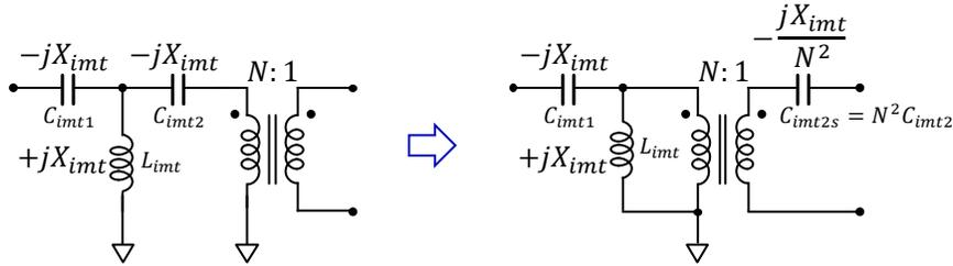
**Figure 6.15:** Magnetics integration in the proposed ICN converter: (a) the three ICN inductors realized using two coupled windings, and (b) the immittance network and transformer combined, with the immittance network inductance realized using the transformer's magnetizing inductance.
