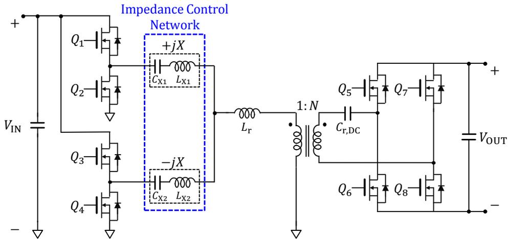
**Figure 5.2:** Impedance control network (ICN) dc-dc converter with its resonant capacitor  $C_r$  moved to the secondary side of the transformer to enable dc blocking.
