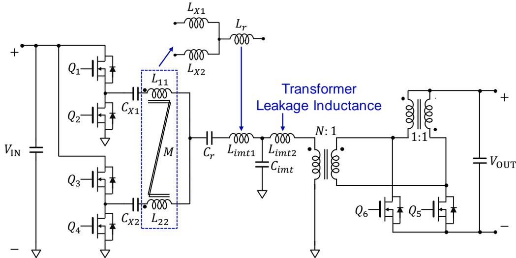
**Figure 7.3:** Realization of immittance network inductances using the coupling of the ICN inductances and the leakage inductance of the transformer.
