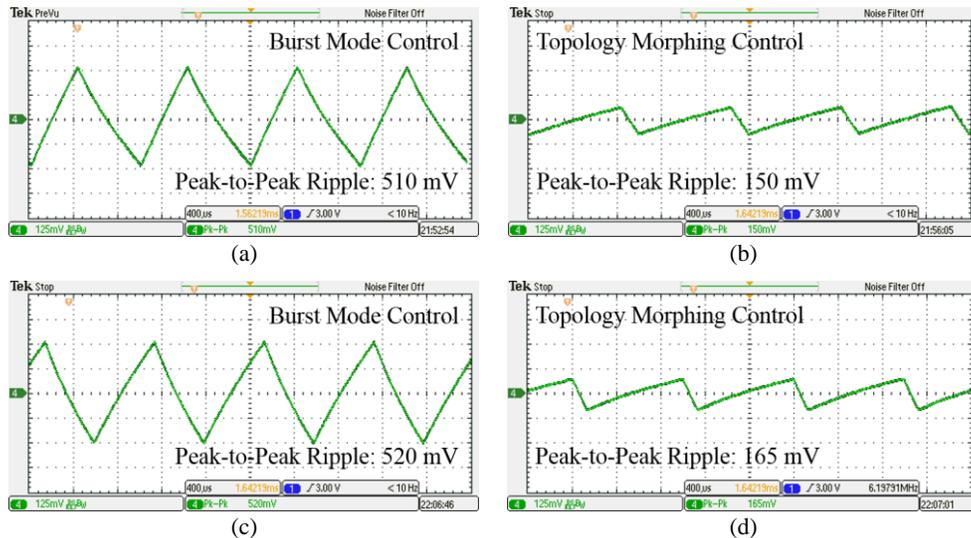
**Figure 5.18:** Output voltage ripple in the prototype ICN converter under the conventional burst-mode control and the proposed topology morphing control at two example operating points: (a), (b)  $V_{IN} = 18$  V,  $V_{OUT} = 12$  V,  $P_{OUT} = 72$  W, and (c), (d)  $V_{IN} = 36$  V,  $V_{OUT} = 12$  V,  $P_{OUT} = 108$  W. These waveforms show the low-frequency ac component  $-\delta v_{OUT}$  of the converter's output voltage.
