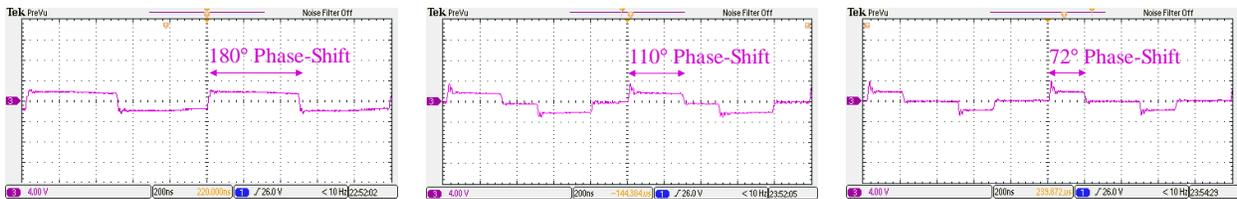
**Figure 7.10:** Rectifier input voltage under rectifier phase-shift control of the final PoL ICN converter prototype.
