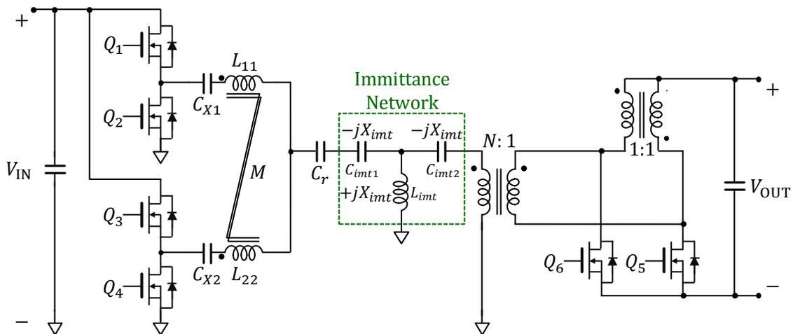
**Figure 6.13:** Impedance control network (ICN) resonant converter utilizing an immittance network to provide voltage step-down.
