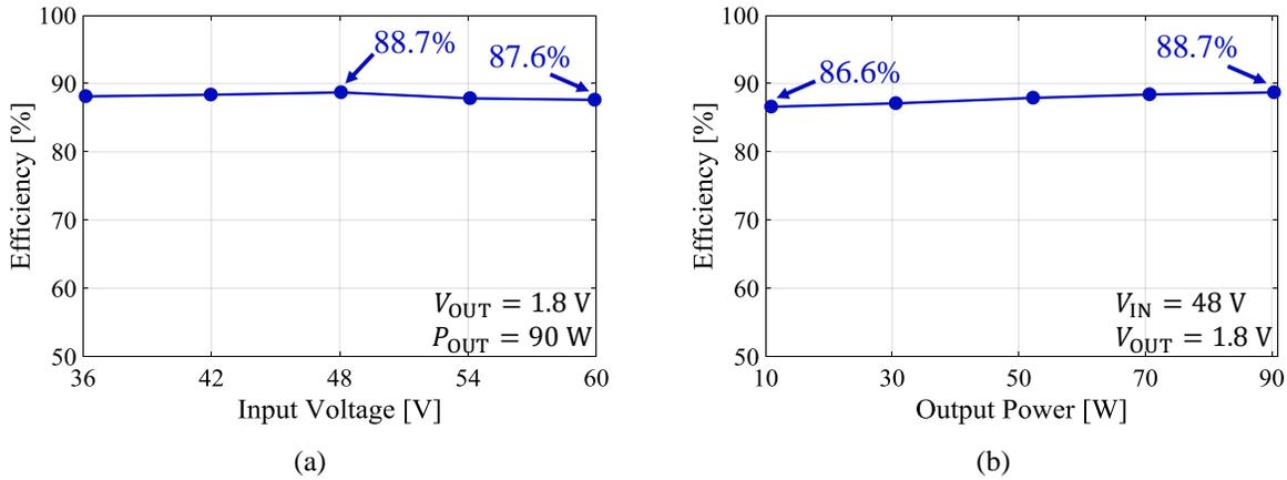
**Figure 6.9:** Measured efficiency of the first PoL ICN converter prototype: (a) as a function of its input voltage at full power ( $P_{OUT} = 90 \text{ W}$ ), and (b) as a function of its output power at its nominal input voltage ( $V_{IN} = 48 \text{ V}$ ). In both (a) and (b), the output voltage  $V_{OUT} = 1.8 \text{ V}$ .
