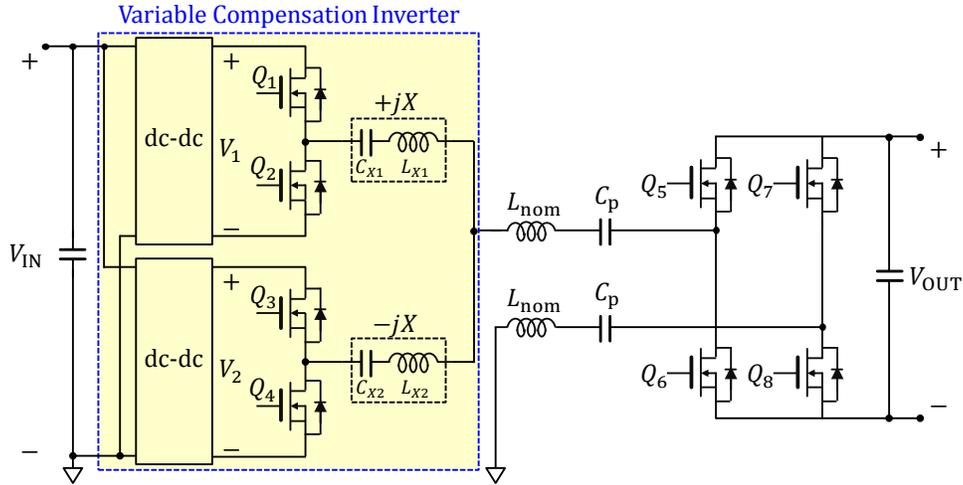
**Figure 9.2:** Example implementation of the variable compensation inverter (VCI) in a capacitive WPT system.
