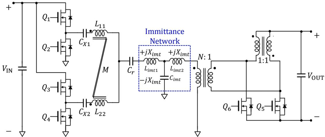
**Figure 7.2:** ICN converter with an alternative implementation of the immittance network.
