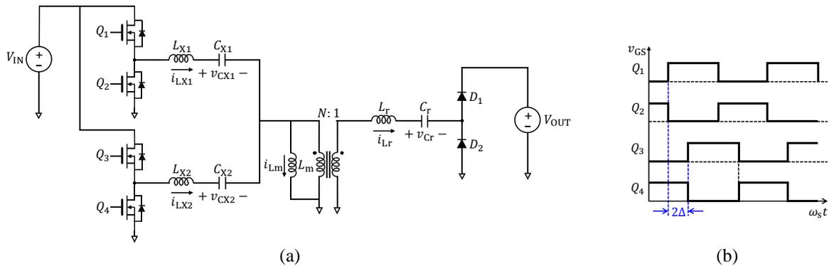
**Figure 2.5:** The impedance control network (ICN) converter of [23]: (a) topology, and (b), switch gating signals demonstrating the phase-shift between the top and bottom inverters.
