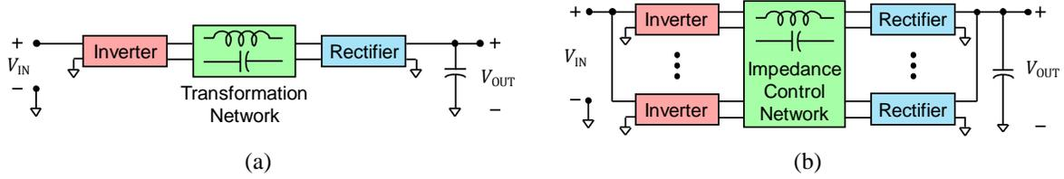
**Figure 1.2:** Architecture of: (a) a conventional resonant dc-dc converter, and (b) an impedance control network resonant dc-dc converter.
