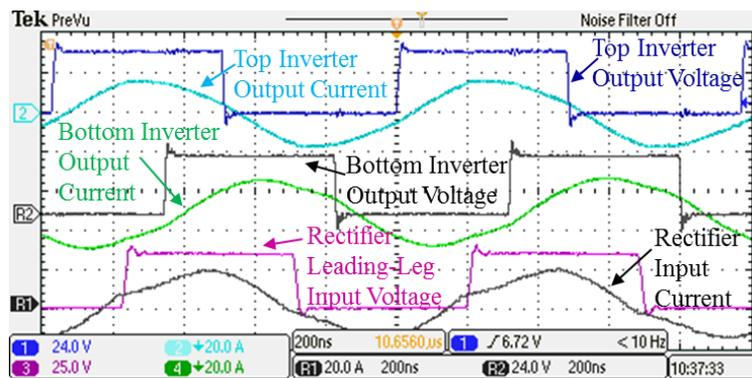
**Figure 3.7:** Measured waveforms for the ICN resonant converter operating at full power (390 W) at 36 V input voltage and 34 V output voltage. Waveforms shown are the output voltage and output current of both (top and bottom) half-bridge inverters, and the input voltage and input current of the leading leg of the rectifier.
