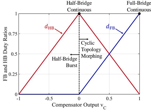
**Figure 5.13:** The full-bridge and half-bridge duty ratios ( $d_{FB}$  and  $d_{HB}$ ) of the proposed topology morphing control as a function of the compensator output  $v_C$ .
