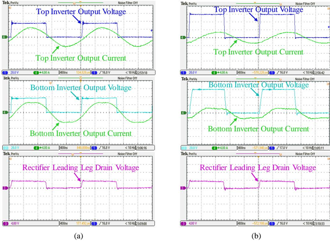
**Figure 6.20:** Inverter and rectifier switching waveforms of the second PoL ICN converter prototype while delivering 90-W output power at: (a)  $V_{IN} = 36\text{ V}$  and  $V_{OUT} = 1.8\text{ V}$ , and (b)  $V_{IN} = 60\text{ V}$  and  $V_{OUT} = 1.8\text{ V}$ .
