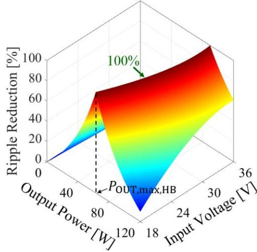
**Figure 5.8:** Reduction in output voltage ripple brought about by the proposed topology morphing control relative to the conventional burst-mode control for the step-down ICN converter design of Table 5.1.
