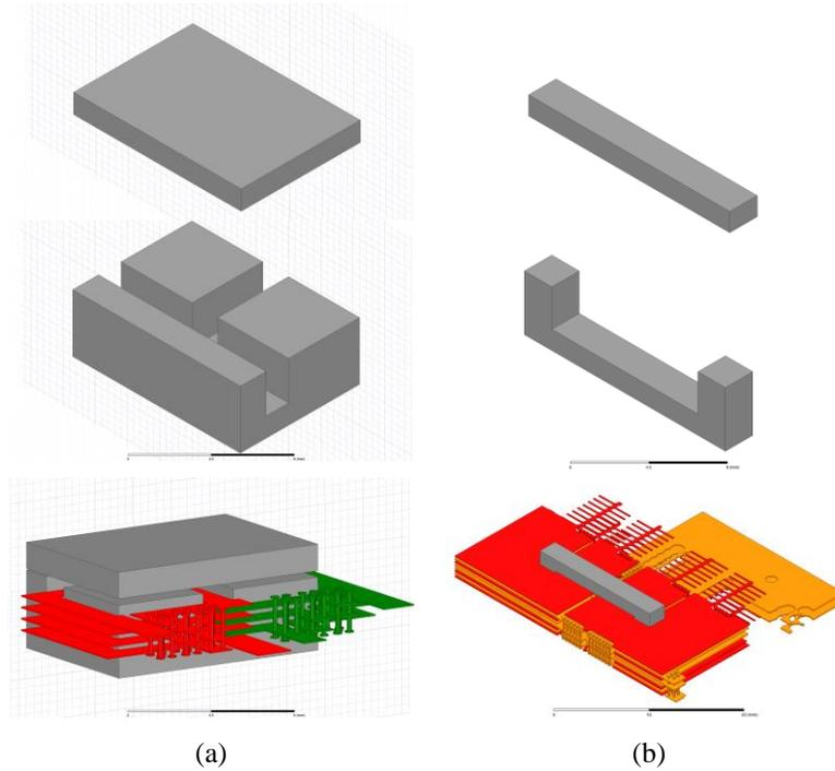
**Figure 7.6:** Ansys HFSS models of the integrated magnetic structures employed in the PoL ICN converter of Fig. 7.5: (a) integrated inductors, and (b) distributed transformer.
