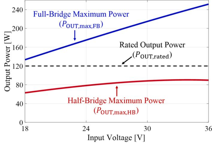
**Figure 5.7:** The full-bridge and half-bridge maximum power levels of an ICN converter designed for an input voltage range of 18 V to 36 V, output voltage of 12 V and rated output power of 120 W.
