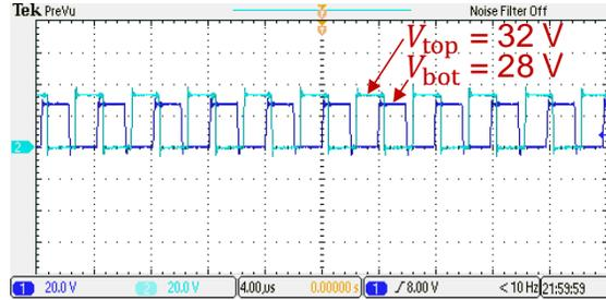
**Figure 6.11:** Output voltages of the two stacked inverters of the first PoL ICN converter prototype, with the converter operating at  $V_{IN} = 48$  V,  $V_{OUT} = 1.8$  V and  $P_{OUT} = 90$  W, demonstrating a mismatch between the two input voltages of the two inverters. The waveform labeled  $V_{top}$  is the output voltage of the top inverter, and the waveform labeled  $V_{bot}$  is the output voltage of the bottom inverter.
