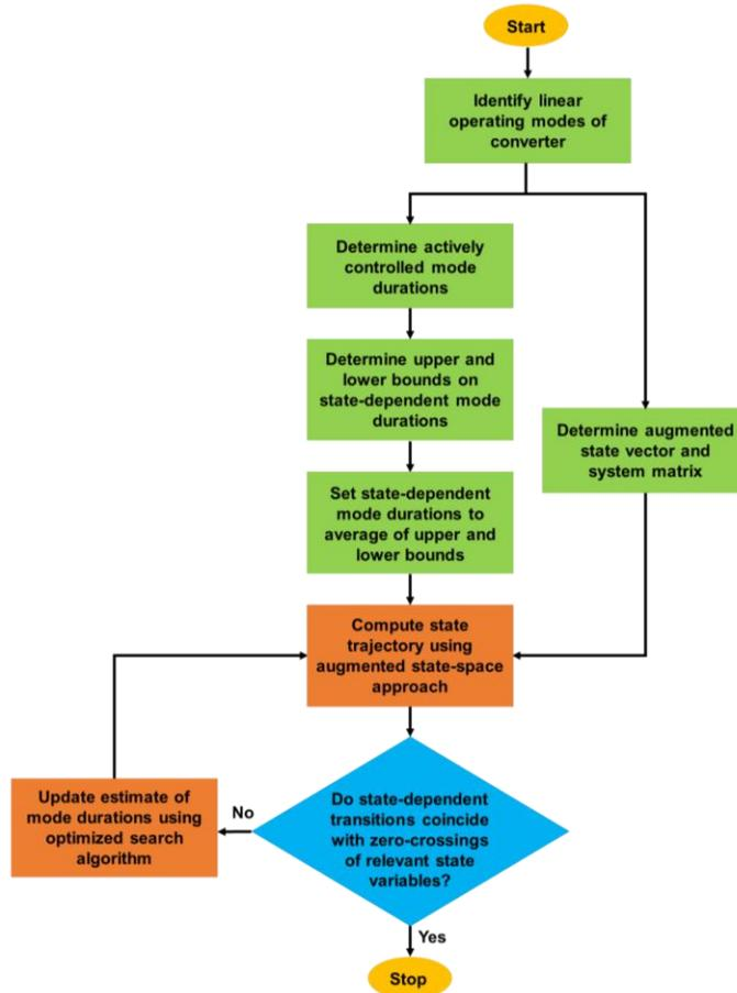
**Figure 2.3:** Flowchart detailing the proposed modeling approach.
