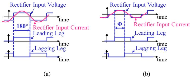
**Figure 7.7:** Rectifier phase-shift control of the PoL ICN converter of Fig. 7.5: (a) full-power operation, and (b) partial-power operation.
