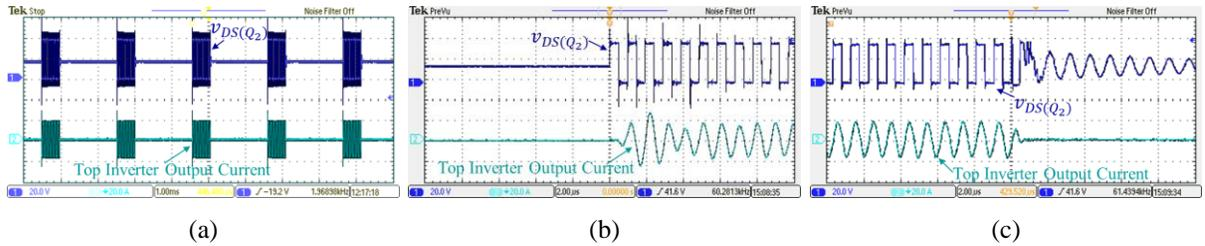
**Figure 3.11:** Burst-mode operation of the ICN converter delivering 25% of the full power at 36 V input voltage and 34 V output voltage. Waveforms shown are the output voltage and output current of the top half-bridge inverter: (a) long timescale showing multiple startup and shutdown sequences, (b) magnified timescale to show the startup dynamics, and (c) magnified timescale to show the shutdown dynamics.
