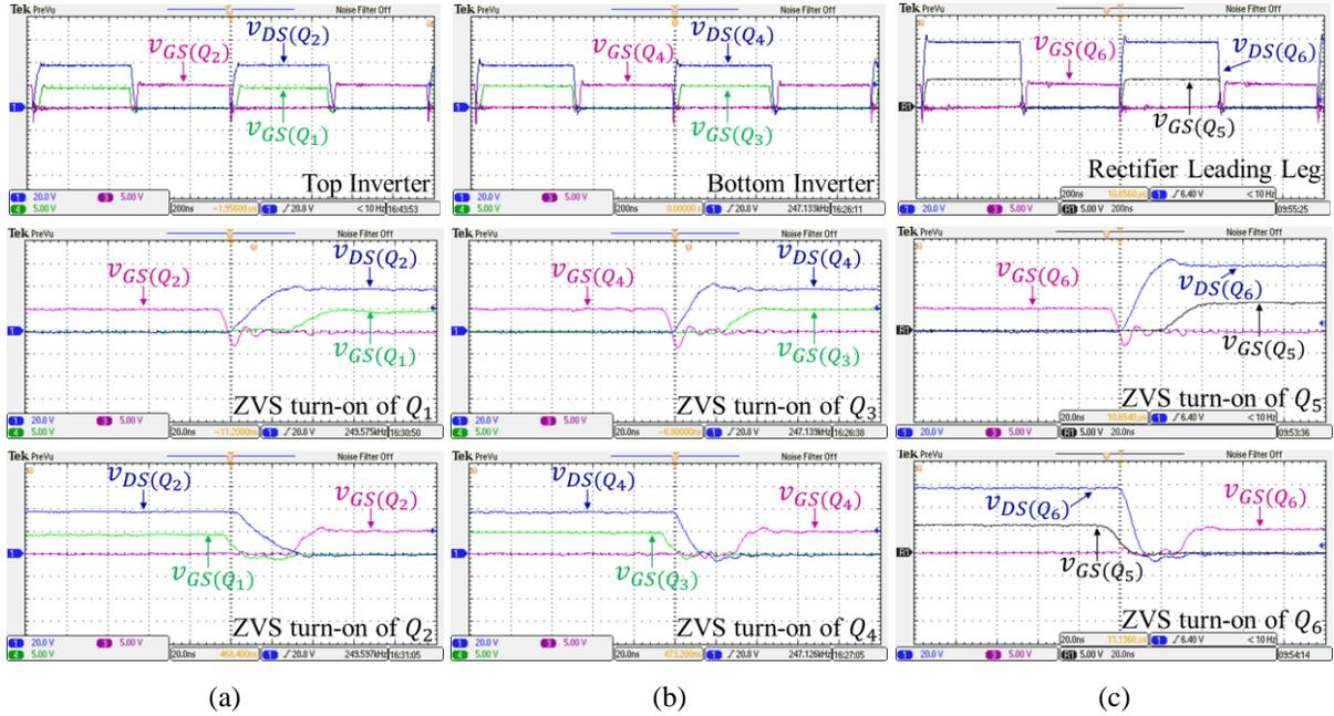
**Figure 3.10:** Measured waveforms confirming ZVS turn-on operation of the ICN resonant converter operating at full power (550 W) at 36 V input voltage and 55 V output voltage. Waveforms shown are the output voltage, output current, and gate signals of: (a) the top inverter, (b) the bottom inverter, and (c) the leading leg of the rectifier.
