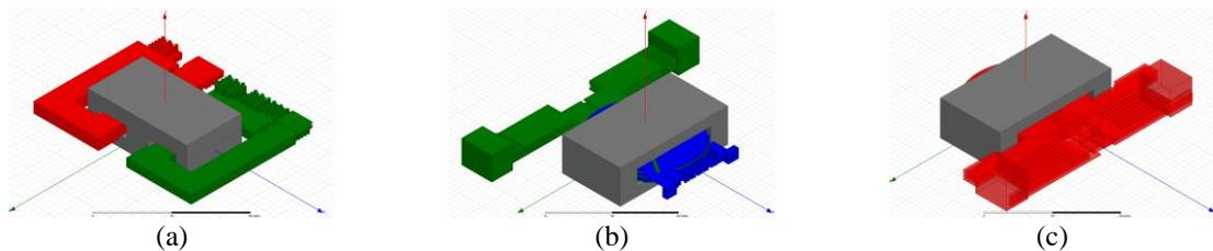
**Figure 6.6:** Maxwell 3D models of the three magnetic components of the PoL ICN converter of Fig. 6.4, with PCB-exported windings including vias and terminal connections: (a) integrated magnetic structure, (b) main transformer, and (c) 1:1 resonant current-doubler transformer.
