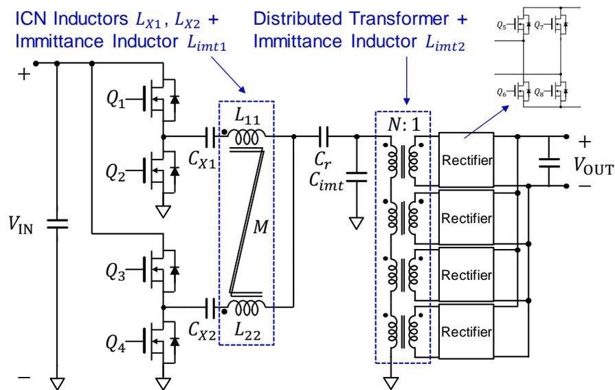
**Figure 7.5:** PoL ICN converter topology with two integrated magnetic structures, one realizing the ICN inductances  $L_{X1}$ ,  $L_{X2}$  and the immittance network inductance  $L_{imt1}$ , and the other realizing a distributed transformer whose leakage inductance is utilized as the immittance network inductance  $L_{imt2}$ .
