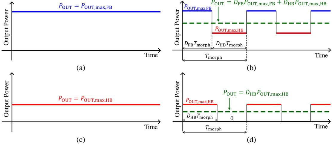
**Figure 5.4:** The four modes of output power regulation in the proposed topology morphing control scheme: (a) full-bridge continuous mode, (b) cyclic topology morphing mode, (c) half-bridge continuous mode, and (d) half-bridge burst-mode.
