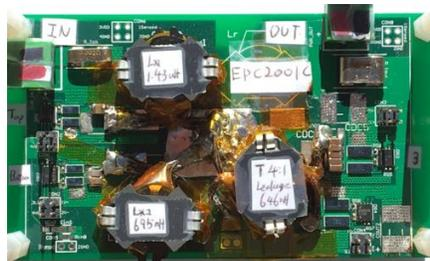
**Figure 5.15:** Photograph of the prototype ICN converter.
