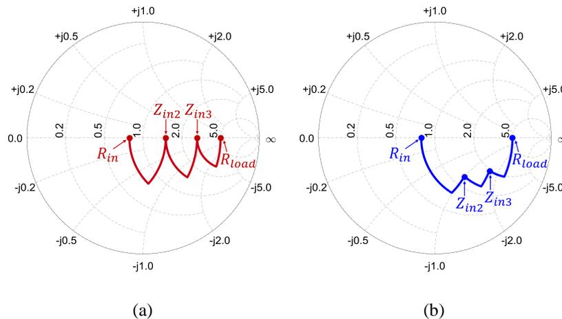
**Figure 8.11:** Smith charts illustrating the impedance transformation provided by the two three-stage networks designed using: (a) conventional approach and (b) proposed approach.  $R_{load}$  denotes the load impedance of the last stage,  $Z_{in3}$  and  $Z_{in2}$  denote the input impedances of the third and second stages, respectively, and  $R_{in}$  denotes the input impedance of the first stage. All impedances are normalized with respect to  $50 \Omega$ .
