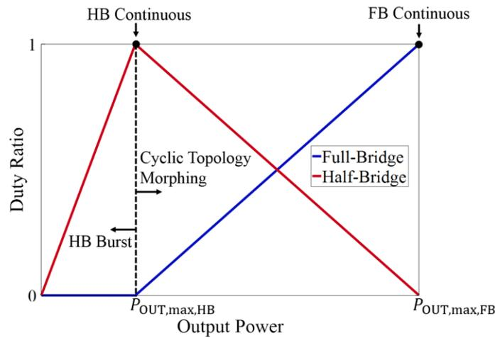
**Figure 5.5:** Duty ratios of full-bridge and half-bridge rectifier operation of the ICN converter across the four modes of the proposed topology morphing control scheme. The half-bridge duty ratio  $D_{HB}$  is shown in red, and the full-bridge duty ratio  $D_{FB}$  in blue.
