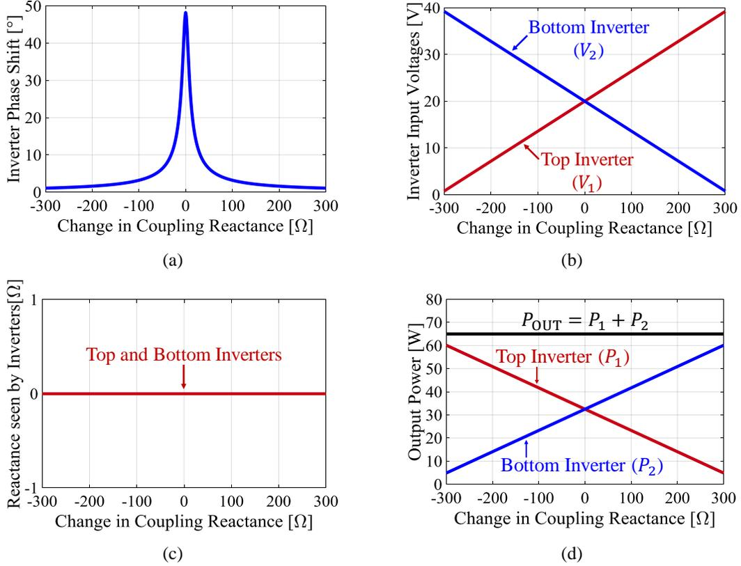
**Figure 9.3:** Variation in operating parameters of the proposed variable compensation inverter (VCI) as the coupling reactance changes: (a) inverter relative phase-shift, (b) input voltages of top and bottom inverters, (c) resultant reactance seen at the outputs of the two inverters, and (d) output power of the two inverters and the total output power.
