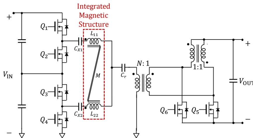
**Figure 6.4:** First PoL ICN converter topology, comprising stacked inverters, a resonant current-doubler rectifier, and a single integrated magnetic structure realizing the three ICN inductances.
