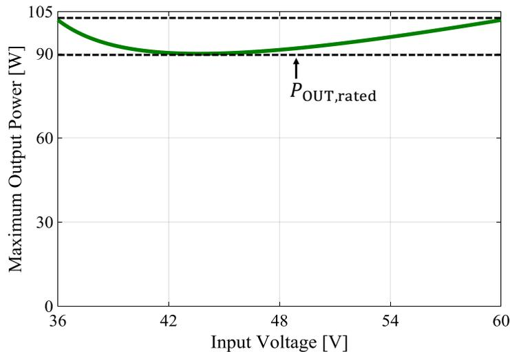
**Figure 6.17:** Maximum output power delivered by the PoL ICN converter of Fig. 6.16 over its input voltage range in a 36V-to-60V input, 1.8-V output, 90-W PoL application.
