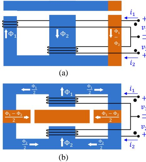
**Figure 4.6:** Alternative implementations of the integrated magnetic structure with: (a) differential flux path on side leg of E core, and (b) horizontally layered flux paths.
