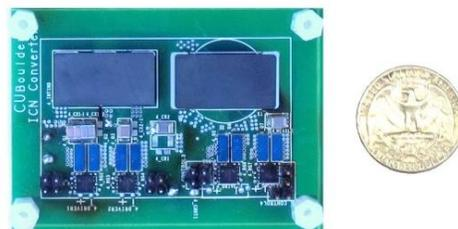
**Figure 4.8:** Photograph of the prototype ICN converter. Also shown for size comparison is a U.S. quarter.
