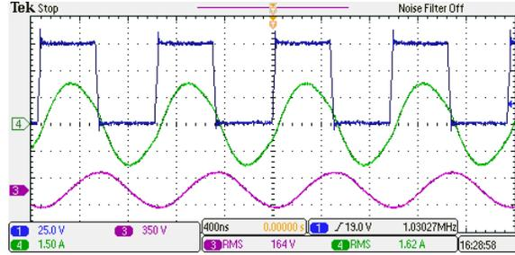
**Figure 8.12:** The inverter output voltage, matching network input current (top waveforms, in blue and green) and load voltage (bottom waveform, in pink) for a single-stage matching network providing a total current gain  $G_{i,tot}$  of 0.4, and operating at an output power of 100 W.
