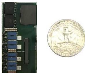
**Figure 7.8:** Photograph of the final 90-W PoL ICN converter prototype. Also shown for size comparison is a U.S. quarter.
