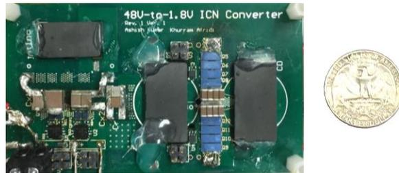
**Figure 6.7:** Photograph of the first 90-W PoL ICN converter prototype. Also shown for size comparison is a U.S. quarter.
