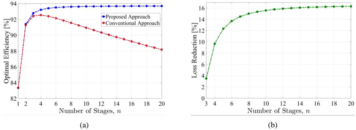
**Figure 8.5:** Comparison of the proposed and the conventional design approach for the multistage matching network of Fig. 2(a) for a total current gain  $G_{i,tot}$  of 0.05, with an inductor quality factor  $Q_L$  of 100: (a) Optimal efficiency as predicted by the proposed and the conventional approach as a function of the number of stages, and (b) Loss reduction achievable with the proposed approach as compared to the optimal 4-stage design of the conventional approach.
