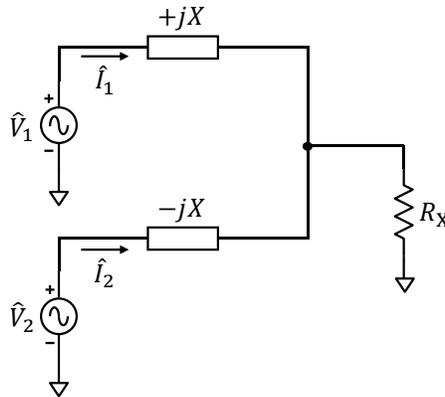
**Figure A.1:** Fundamental-frequency model of the ICN converter.
