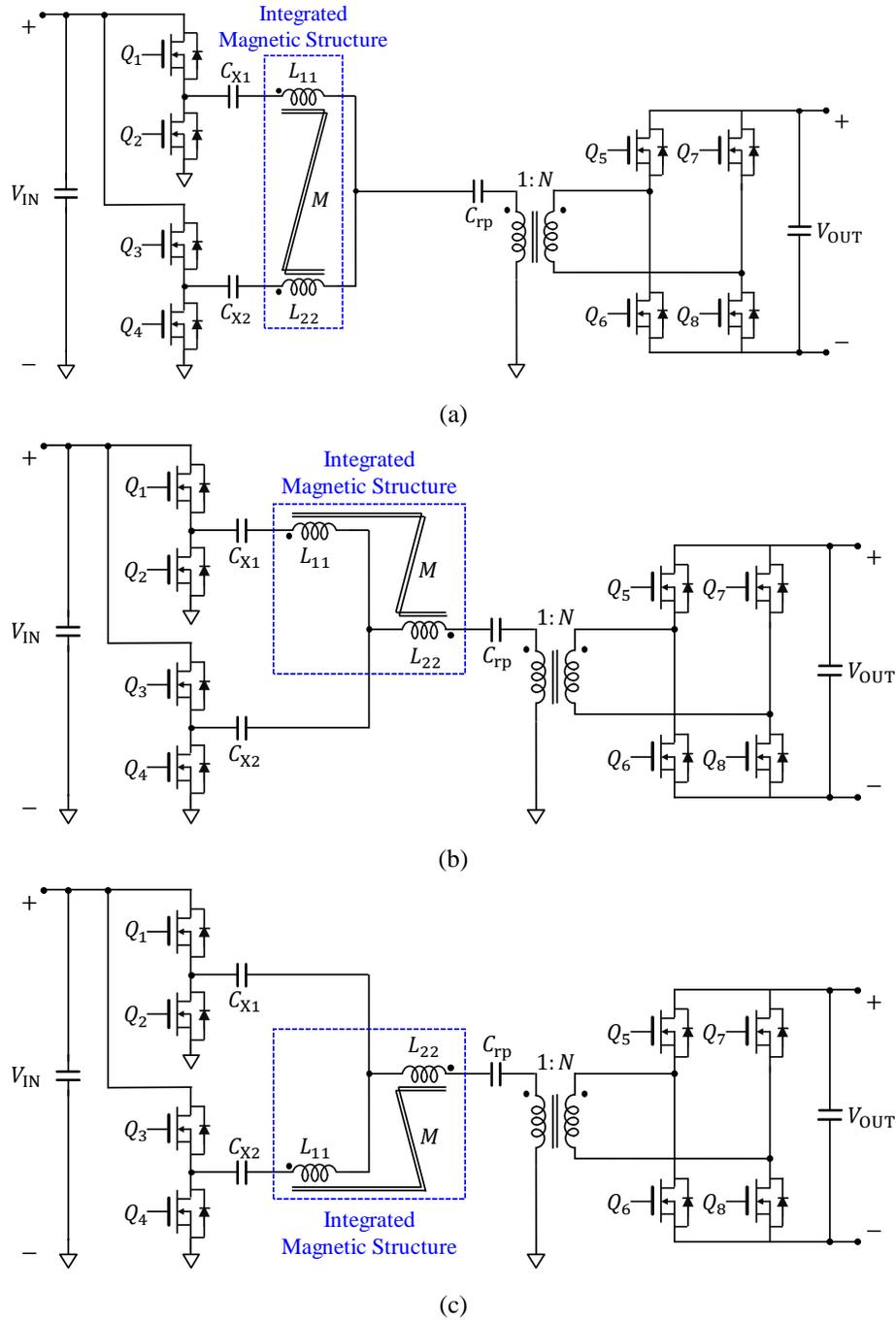
**Figure 4.4:** The three ICN converter topologies resulting from the coupling configurations of Fig. 4.3.
