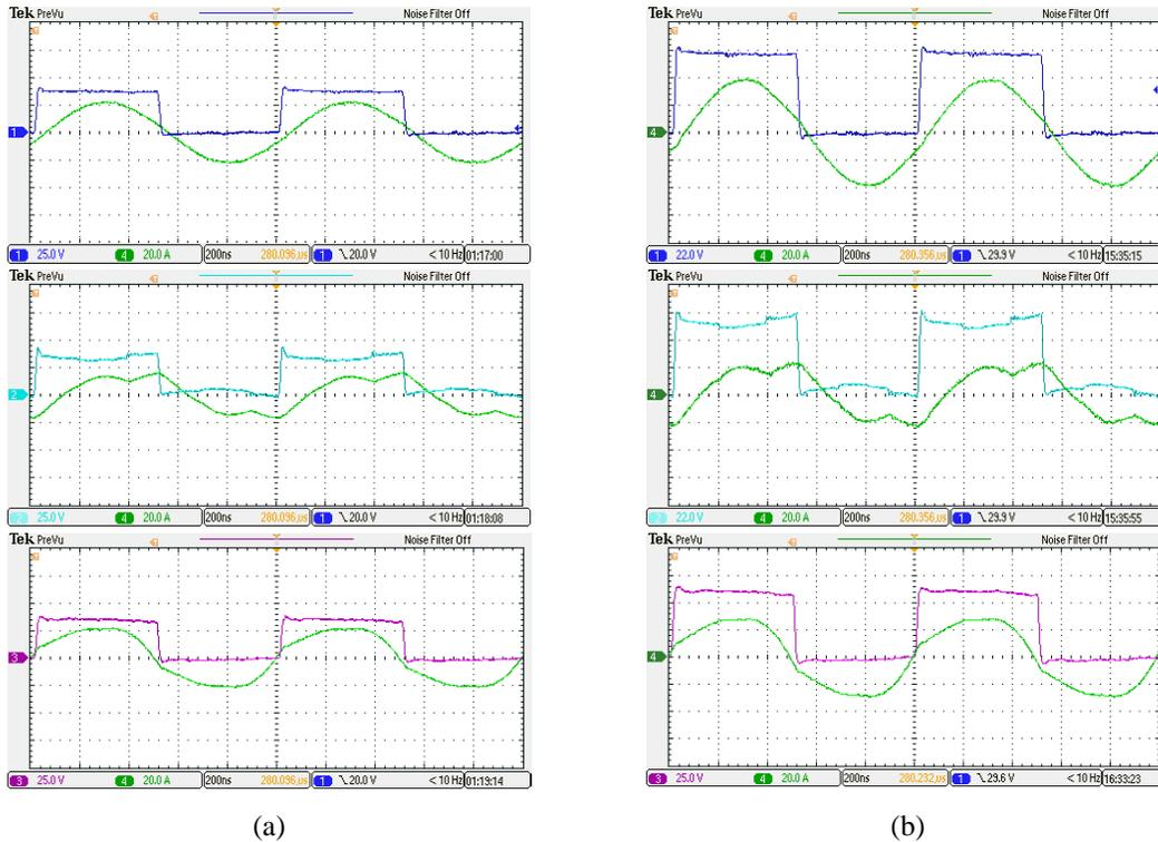
**Figure 4.9:** Inverter and rectifier switching waveforms of the prototype ICN converter while delivering full power at: (a)  $V_{IN} = 36$  V,  $V_{OUT} = 34$  V and (b)  $V_{IN} = 60$  V,  $V_{OUT} = 55$  V. The waveforms shown in (a) and (b) are, from top to bottom, the output voltage and current of the top inverter, the output voltage and current of the bottom inverter and the input voltage and current of the leading leg of the rectifier.
