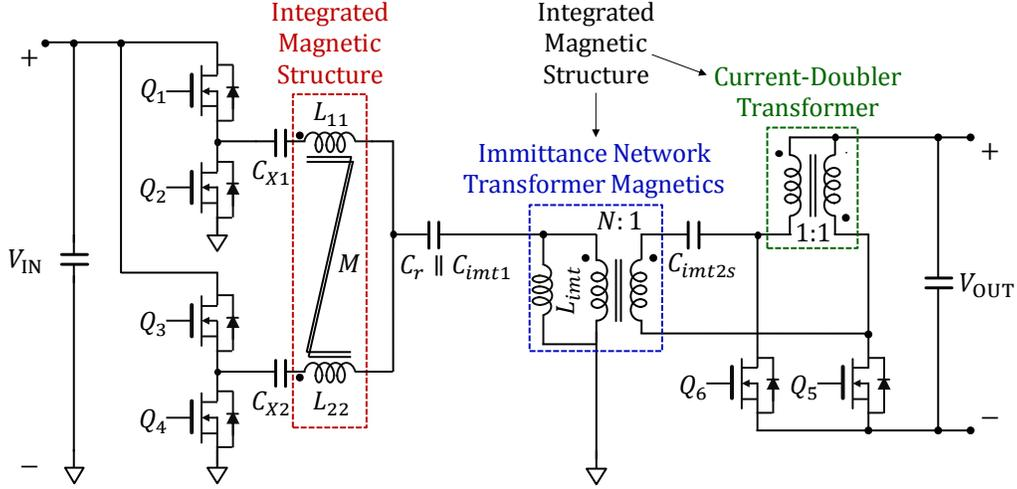
**Figure 6.16:** Second PoL ICN converter topology, comprising an immittance network transformer and a resonant current-doubler rectifier, with all magnetic components combined into two integrated magnetic structures. Note that one of the capacitances of the immittance network,  $C_{imt1}$ , is series combined with the resonant capacitor  $C_r$  and implemented as a single capacitor.
