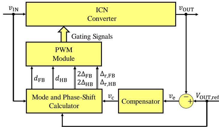
**Figure 5.12:** Closed-loop control architecture for multimode topology morphing control of ICN converter.
