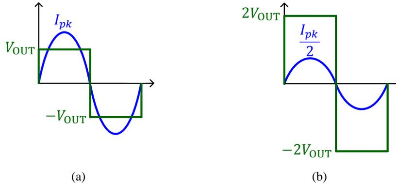
**Figure 6.3:** Transformer secondary voltage and fundamental-frequency current with: (a) full-bridge rectifier, and (b) resonant current-doubler rectifier, with both rectifier operating at the same output power level. Compared to the full-bridge rectifier, the current-doubler rectifier doubles the transformer secondary voltage by providing a voltage step-down of 2:1, and halves the transformer secondary current.
