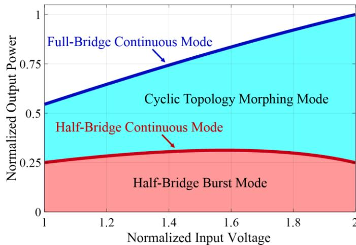
**Figure 5.3:** The four modes of the proposed topology morphing control scheme. Here the output power of the ICN converter (the y-axis) is normalized with respect to the maximum power the converter can deliver with a full-bridge rectifier, and the input voltage (the x-axis) is normalized with respect to the minimum input voltage of the converter.
