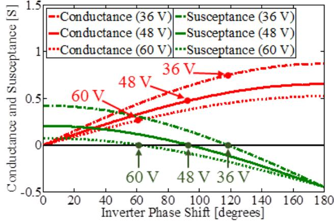
**Figure 3.2:** Effective conductance and susceptance seen by the two inverters of the ICN converter of Fig. 3.1 as a function of the inverter phase-shift, for three input voltage values: 36 V, 48 V and 60 V, and for an output voltage of 34 V.
