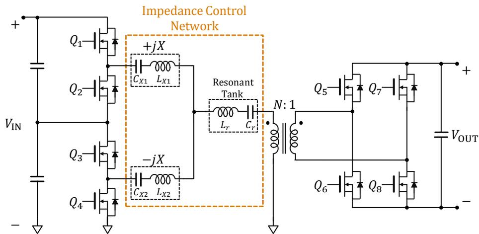
**Figure 6.1:** ICN resonant converter with stacked inverters.
