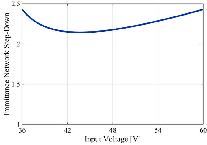
**Figure 6.14:** Voltage step-down provided by an immittance network in a 90-W POL ICN converter with an input voltage range of 36 V–60 V and an output voltage of 1.8 V. Here, the immittance network reactance  $X_{imt}$  is chosen to be 4  $\Omega$ .
