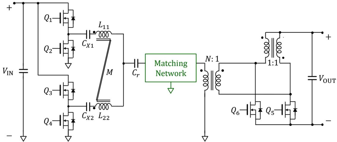
**Figure 6.12:** Impedance control network (ICN) resonant converter utilizing a matching network to provide voltage step-down.
