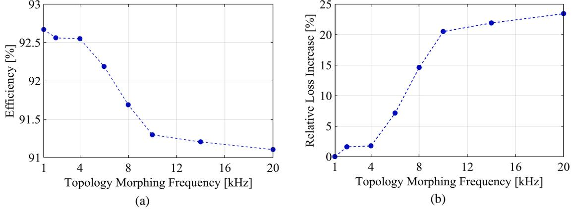
**Figure 5.21:** Performance of prototype ICN converter as a function of topology morphing frequency when operating in the cyclic topology morphing mode of the proposed control approach, at  $V_{IN} = 18$  V,  $V_{OUT} = 12$  V and  $P_{OUT} = 72$  W: (a) efficiency, and (b) percentage increase in losses relative to the losses at 1-kHz topology morphing frequency.
