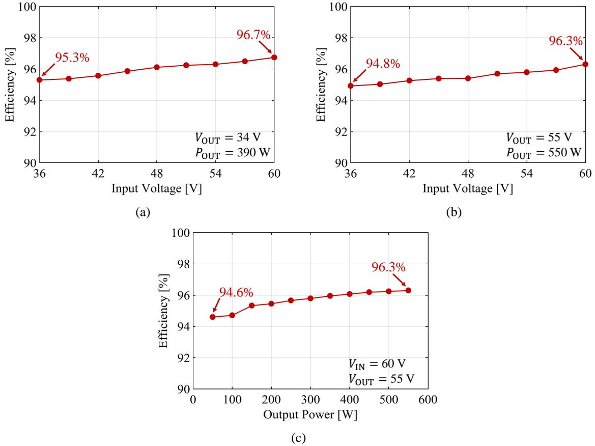
**Figure 4.10:** Measured efficiency of the prototype ICN converter across variations in: (a) input voltage at its minimum output voltage of 34 V; (b) input voltage at its maximum output voltage of 55 V; and (c) output power with an input voltage of 60 V and output voltage of 55 V.
