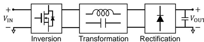
**Figure 2.1:** Architecture of a typical resonant dc-dc converter.
