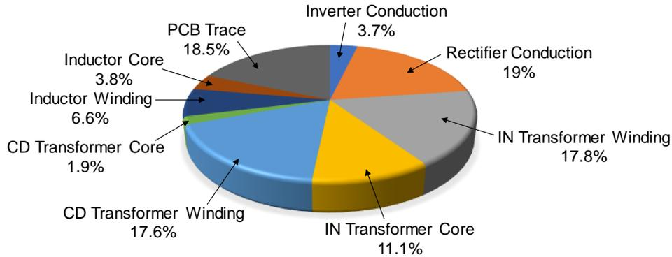
**Figure 6.22:** Theoretically predicted loss breakdown of the first PoL ICN converter prototype, operating at  $V_{IN} = 36$  V,  $V_{OUT} = 1.8$  V and  $P_{OUT} = 90$  W. Here, “IN” is an abbreviation for immittance network, and “CD” is an abbreviation for current-doubler.
