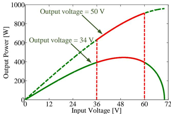
**Figure 3.3:** Variation in output power as a function of input voltage for the ICN converter of Fig. 3.1 operated with the phase-shift between the two inverters controlled to provide zero effective susceptance of the inverters.
