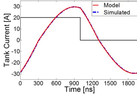
**Figure 2.4:** Comparison between modeled and simulated tank currents of a half-bridge series resonant converter operating in steady state with 200 V input voltage, 100 V output voltage and 500 kHz switching frequency. Also shown for reference is a scaled version of the inverter output voltage (in black).
