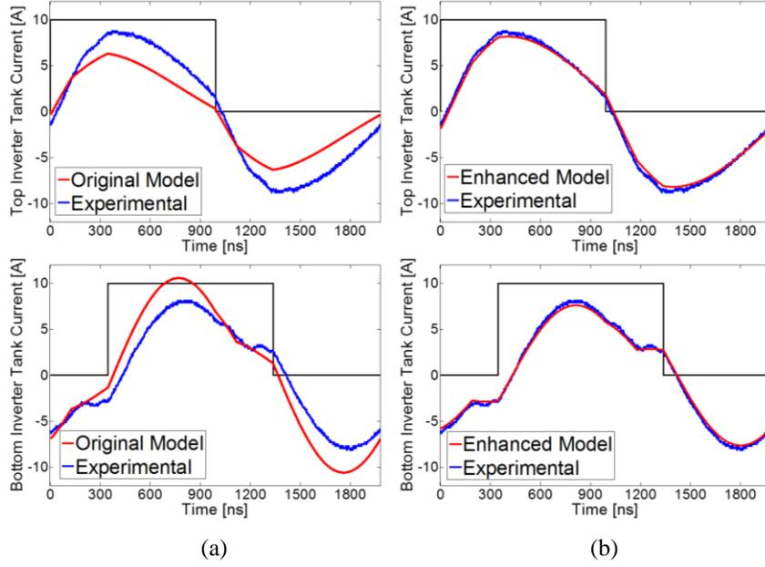
**Figure 2.7:** Comparison of modeled and experimental inverter tank currents of the ICN converter operating at an input voltage of 40 V and output voltage of 250 V: (a) with ideal model, and (b) with model including diode non-ideality. Also shown (in black) are scaled versions of the inverter output voltages.
