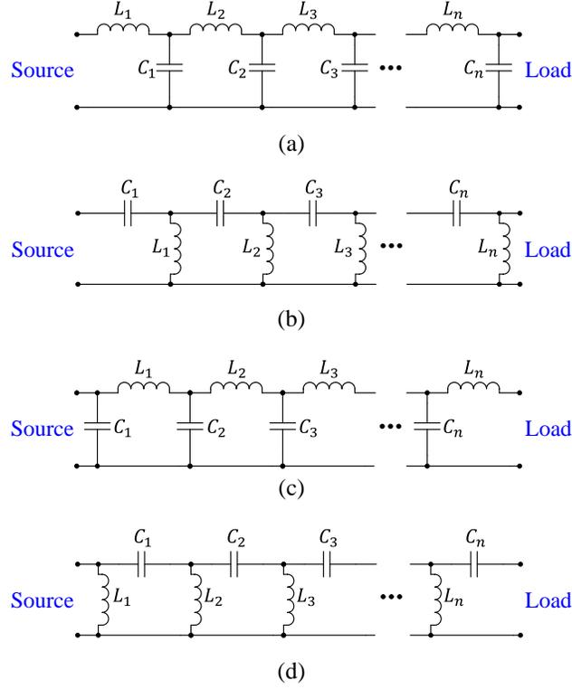
**Figure 8.2:** Four types of multistage matching networks constructed by cascading the corresponding L-section stages of Fig.1. The multistage networks shown in (a) and (b) are appropriate for stepping-up voltage (that is, for total current gains  $G_{i,tot} \leq 1$ ), while those in (c) and (d) are suitable for stepping-up current ( $G_{i,tot} \geq 1$ ).
