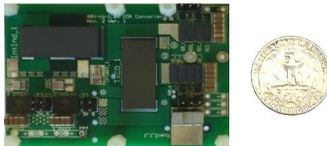
**Figure 6.19:** Photograph of the second 90-W PoL ICN converter prototype. Also shown for size comparison is a U.S. quarter.
