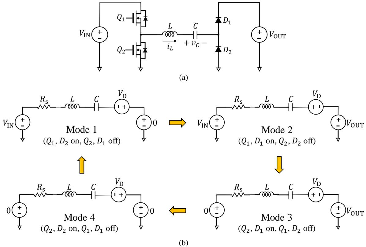
**Figure 2.2:** A half-bridge input, half-bridge output series resonant converter: (a) topology and (b) equivalent circuit in each linear operating mode.
