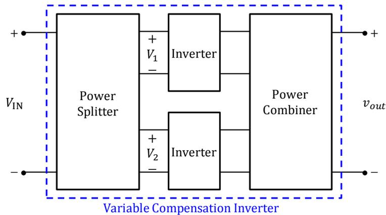
**Figure 9.1:** Architecture of the proposed variable compensation inverter (VCI).
