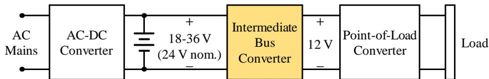
**Figure 5.14:** Application of the proposed ICN converter as an intermediate bus converter in a power distribution system for telecommunications equipment.
