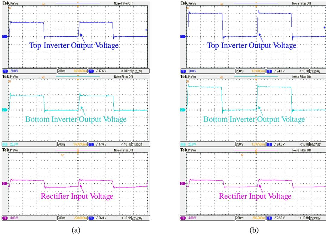
**Figure 7.9:** Inverter and rectifier switching waveforms of the final PoL ICN converter prototype while operating at: (a)  $V_{IN} = 36$  V and  $V_{OUT} = 1.8$  V, and (b)  $V_{IN} = 60$  V and  $V_{OUT} = 1.8$  V.
