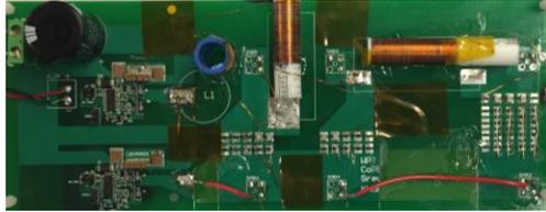
**Figure 8.8:** Photograph of the prototype test circuit comprising a full-bridge inverter, a three-stage L-section matching network, and a  $250\ \Omega$  RF load resistor.
