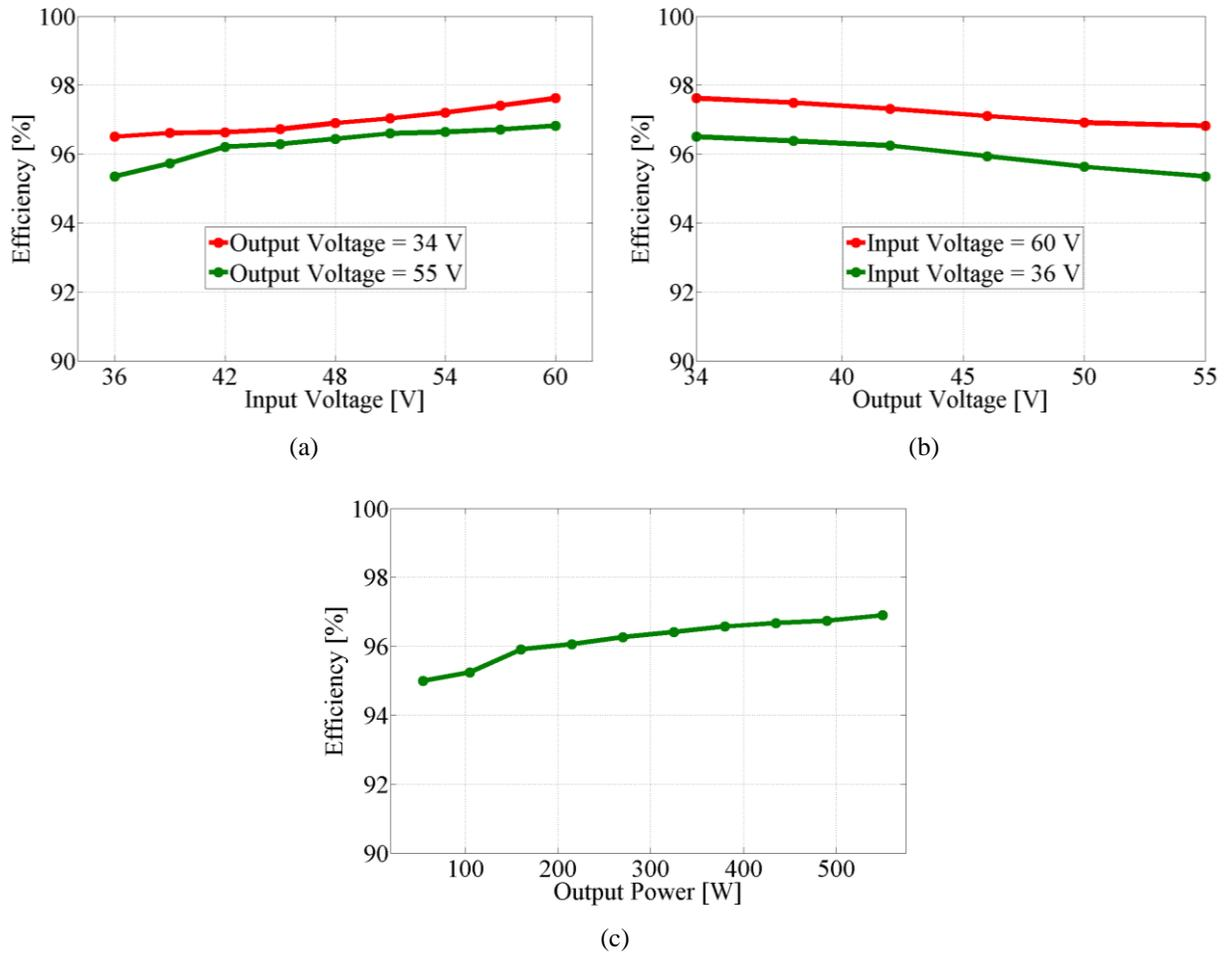
**Figure 3.12:** Measured efficiency of the ICN resonant converter across variations in: (a) input voltage at output voltages of 34 V and 55V at full power; (b) output voltage with input voltages of 36 V and 60 V at full power; and (c) output power with input voltage of 60 V and output voltage of 50 V.
