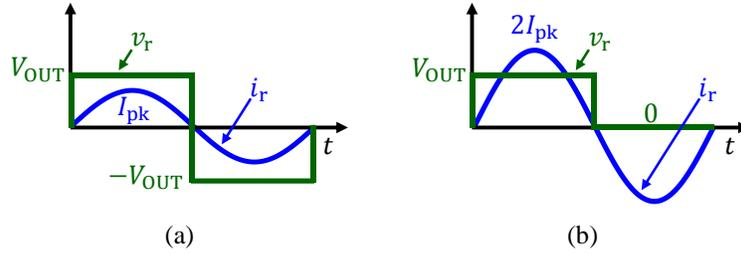
**Figure 5.10:** Fundamental-frequency rectifier input voltage  $v_r$  and current  $i_r$  for a: (a) full-bridge rectifier, and (b) half-bridge rectifier, with both rectifiers operating at the same output power (averaged over one switching period). As can be seen, the half-bridge rectifier in (b) transmits zero power during the second half of the switching period (since its input voltage is 0), resulting in twice the peak current compared to the full-bridge rectifier in (a).
