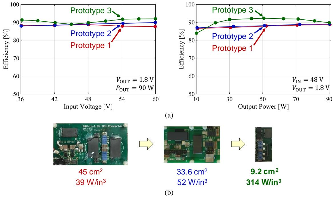
**Figure 7.12:** Performance comparison of the three PoL ICN converter prototypes developed in this thesis: (a) efficiency comparison, and (b) power density comparison.
