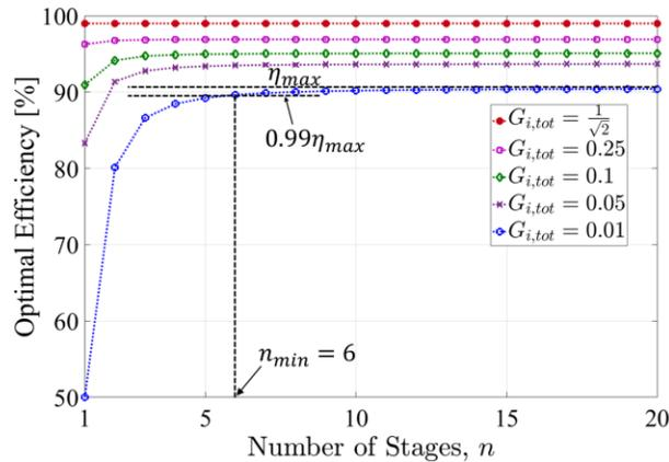
**Figure 8.3:** Optimal efficiency of the multistage network of Fig. 2(a) as a function of the number of stages for various total current gains  $G_{i,tot} \leq \frac{1}{\sqrt{2}}$ , as predicted by the proposed design approach. It can be seen that for this range of total current gains, the optimal efficiency increases monotonically with the number of stages, approaching an asymptotic maximum for each value of  $G_{i,tot}$ .
