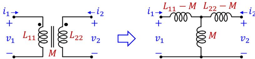
**Figure 4.2.** Modeling of two coupled windings by a T-network of inductors.
