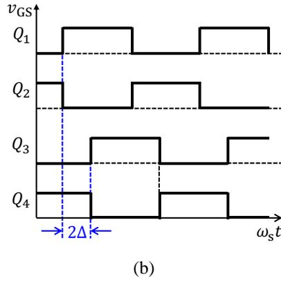
**Figure 3.1:** Impedance control network (ICN) resonant dc-dc converter: (a) topology, and (b) inverter gating signals.
