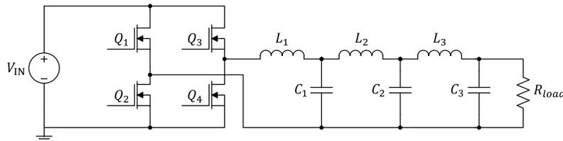
**Figure 8.7:** Prototype circuit to test matching network efficiency. A full-bridge inverter converts a dc voltage into high-frequency ac, which is fed into a three-stage L-section matching network loaded by a 250  $\Omega$  resistance.
